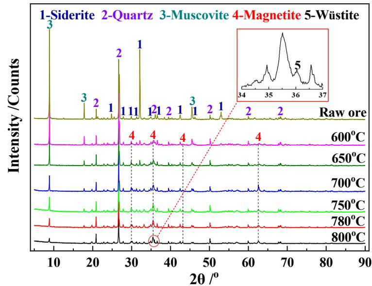
Figure 5. XRD patterns of the roasted ore.
