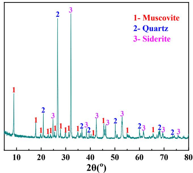
**Figure 1.** X-ray diffraction pattern of Daxigou siderite.
