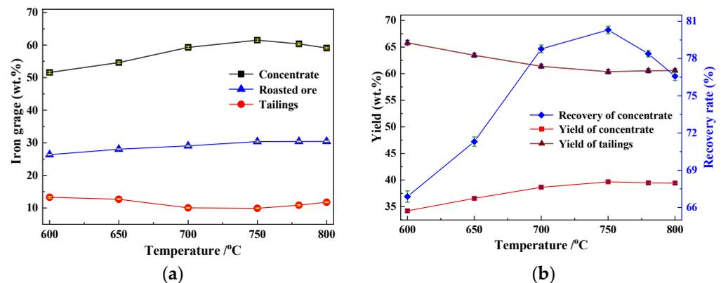
Figure 6. (a) Iron grade and (b) yield and recovery of samples.
