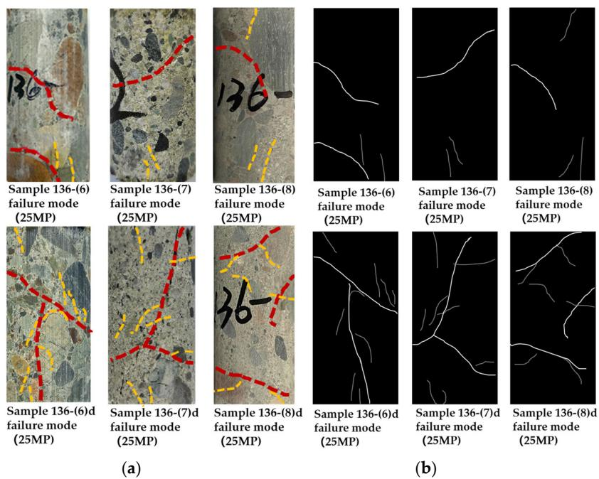
**Figure 13.** Failure modes of Mahu conglomerate under 25 MPa confining pressure. (a) Rock samples, (b) failure modes.
