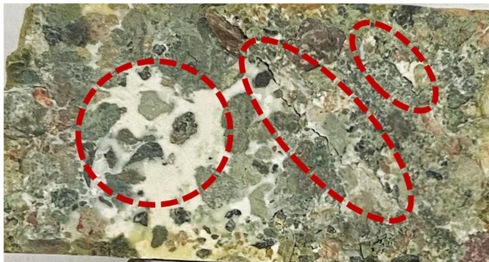
**Figure 6.** Acid marks and obvious fractures after acidizing.
