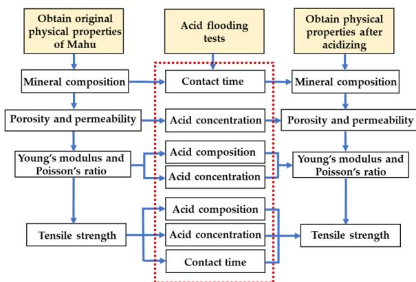
**Figure 2.** Workflow process chart of acidizing factors study.
