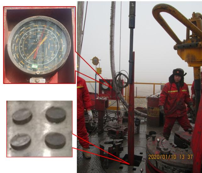
**Figure 20.** Setting experiment of inserted tooth slip sidetracking packer.
