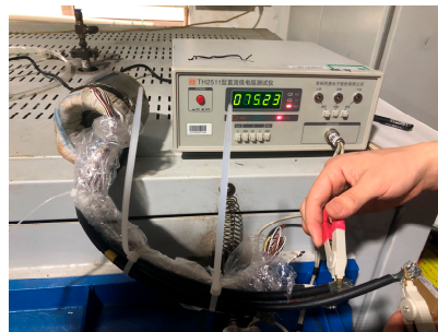
Figure 6. Photo of motor DC resistance test.
