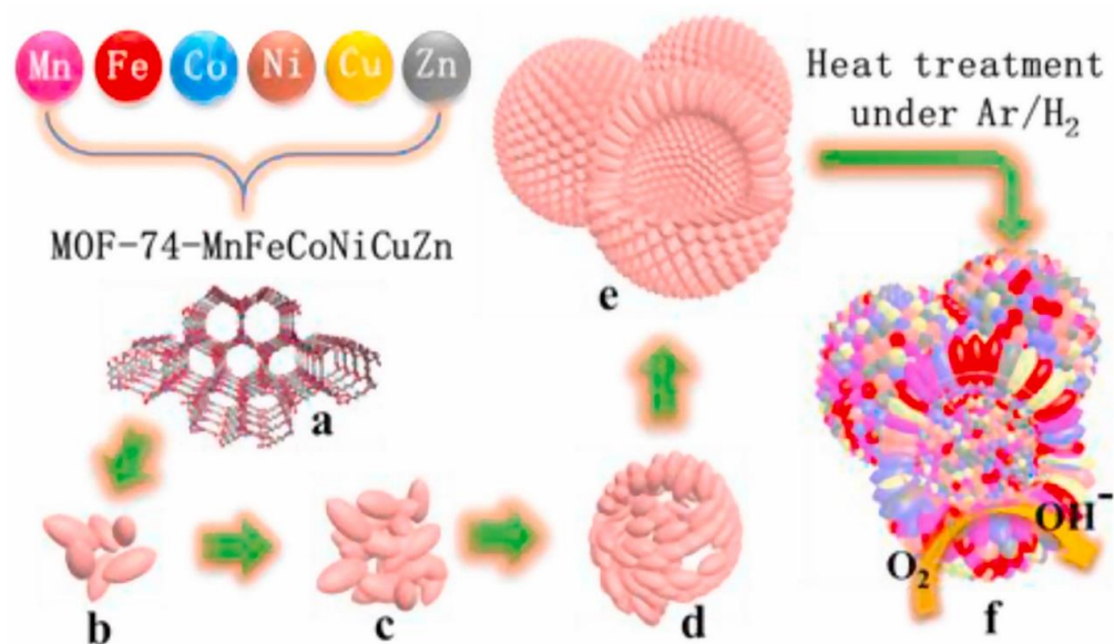
Figure 21. Schematic diagram of porous hollow high-entropy alloy catalyst production. (a) Crystal structure of MOF-74-H. (b) Small number of MOF particle aggregated. (c) Large number of MOF
