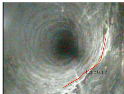
Longitudinal crack at 14.37 m of measuring hole
