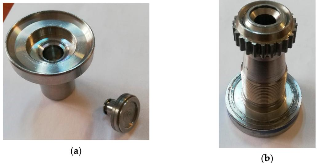
**Figure 2.** Pressure valve subassemblies: (a)—the plate assembly; (b)—the seat assembly.
