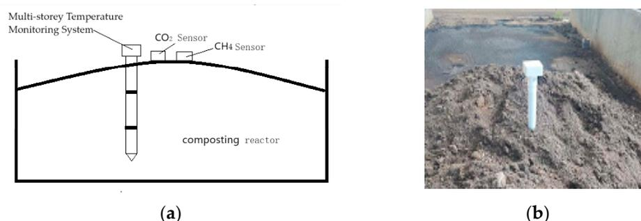
**Figure 1.** The online monitoring system for the composting reactor parameters. (a) Schematic of the temperature and CO<sub>2</sub> concentration; (b) multi-storey temperature monitoring system for the composting reactor.
