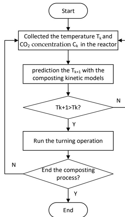
**Figure 2.** The process of the control strategy used for the turning operation for the composting reactor.
