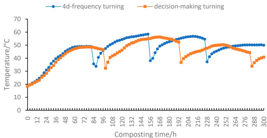
**Figure 6.** The temperature changes for 4d turning frequency and turning using the decision-making method.
