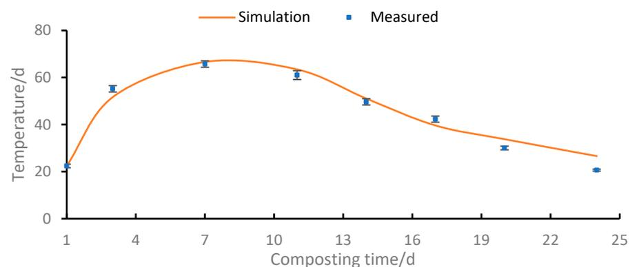
**Figure 5.** The simulation results for the temperature in the composting reactor.
