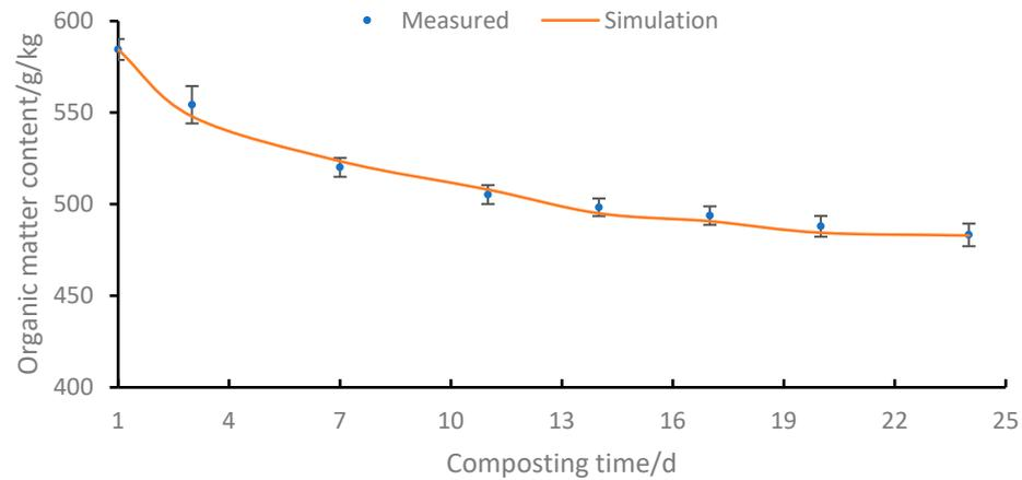
**Figure 4.** The simulation results of organic matter content in the composting reactor.
