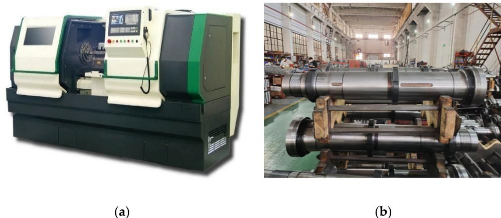
**Figure 7.** The universal CNC machine tool CY-K510 and its spindle NPH02051. (a) The universal CNC machine tool CY-K510; (b) the spindle NPH02051 of CY-K510.
