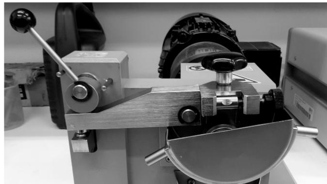
**Figure 2.** Reichert Friction and Wear Tester with used test roller.
