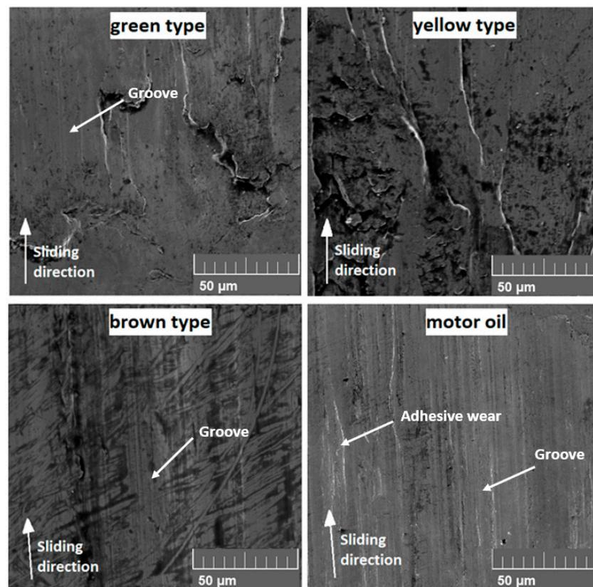
Figure 7. SEM images of the pin after Reichert test for different types of coconut oil and motor oil.
