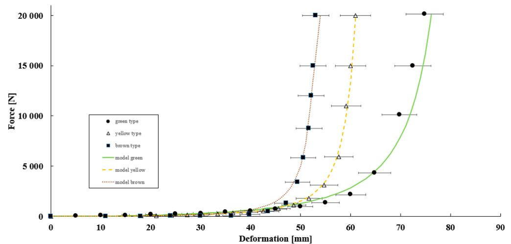
**Figure 3.** Measured values and fitted model for different types of coconuts with displayed amounts of coefficients of variation.
