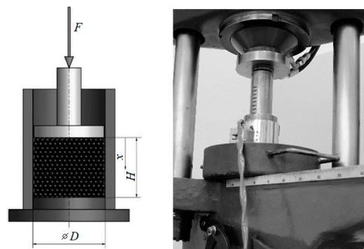
**Figure 1.** Schematic of a pressing vessel with a plunger diameter of 60 mm and the compression test.
