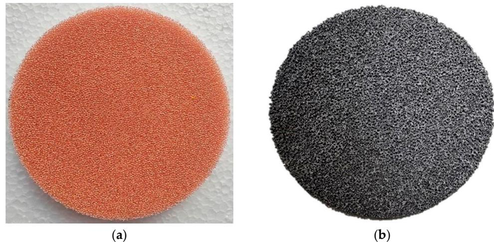
**Figure 6.** Test materials that do not meet the two basic assumptions: (a) copper foam; (b) porous Sic ceramics.
