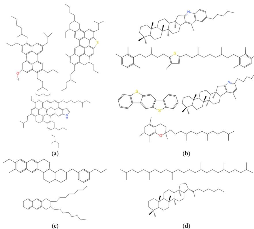
**Figure 7.** Twelve molecular structures of four-component asphalt: (a) Asphaltenes; (b) Polar Aromatics; (c) Naphthene Aromatics; (d) Saturates.
