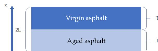
**Figure 2.** The boundary conditions of the diffusion system. ( $L$  was the boundary size of each part).
