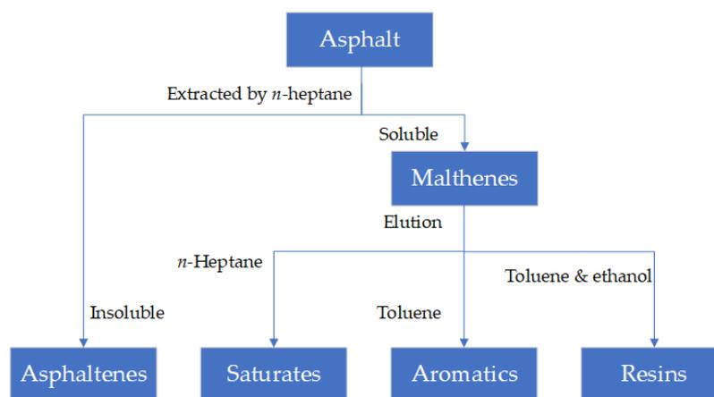
**Figure 4.** The main process of separating asphalt [30].
