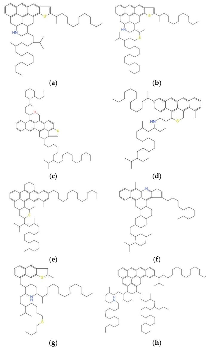
**Figure 5.** Main structures of asphalt average molecular model: (a) AAA-1; (b) AAK-1; (c) AAAF-1; (d) AAB-1; (e) AAC-1; (f) AAG-1; (g) AAD-1; (h) AAM-1.
