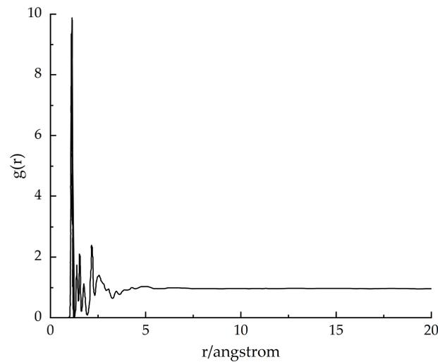
**Figure 10.** The radial distribution function of atoms in the asphalt model [72].
