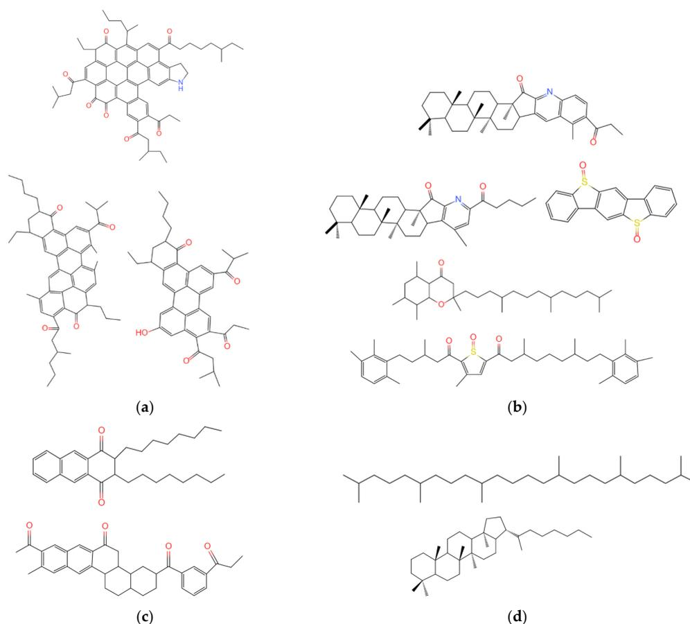
**Figure 9.** Main molecular structure of aged asphalt: (a) Aged asphaltene; (b) Aged polar aromatics; (c) Aged naphthene aromatic; (d) Aged saturate.
