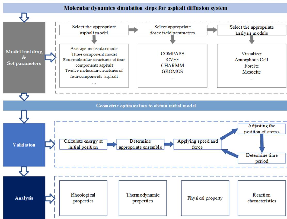
**Figure 3.** Basic steps for molecular dynamics simulation of asphalt diffusion systems.
