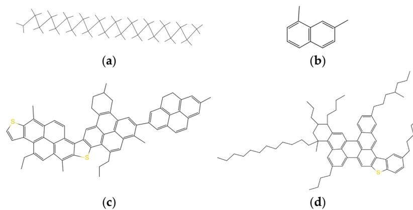
**Figure 6.** Three-component model molecular structure: (a) Saturate; (b) Resin; (c) Asphaltene I; (d) Asphaltene II.
