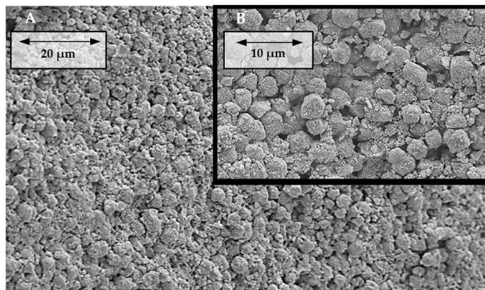
Figure 9. SEM image of the starting 13X zeolite: magnifications of  $1000\times$  (A) and  $3000\times$  (B).
