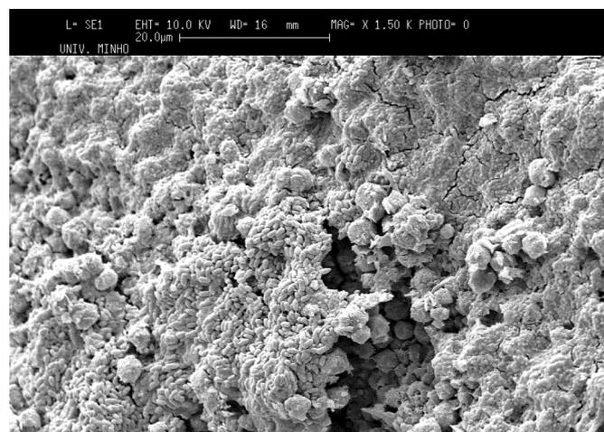
Figure 10. SEM image of *R. viscosum* biofilm supported on 13X zeolite (magnification of  $1500\times$ ).
