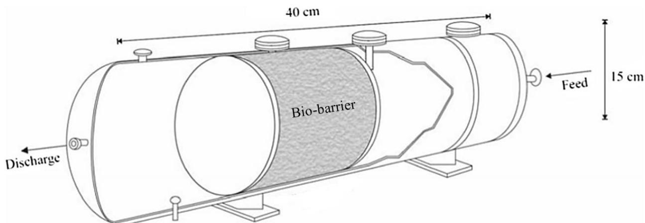
Figure 1. Permeable bio-barrier reactor design.
