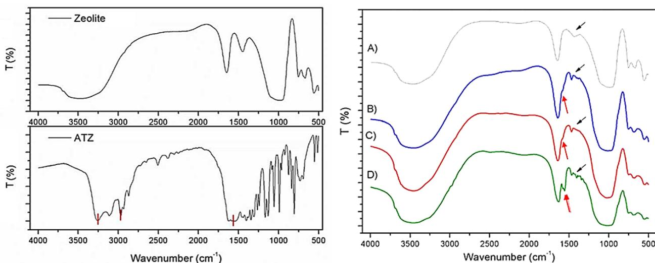
**Figure 8.** FTIR spectra of the starting 13X zeolite and atrazine (left) and of zeolite samples obtained after batch and reactor experiments (right): (A) permeable barrier reactor; (B) biosorption by bacteria/zeolite; (C) biosorption by adapted biofilm/zeolite; (D) adsorption with zeolite. Black and red arrows indicate bands centered at  $1300\text{ cm}^{-1}$  and  $1550\text{ cm}^{-1}$ , respectively.
