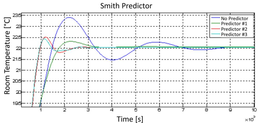
Figure 20. Control results: Smith Predictor architecture performances (CV).
