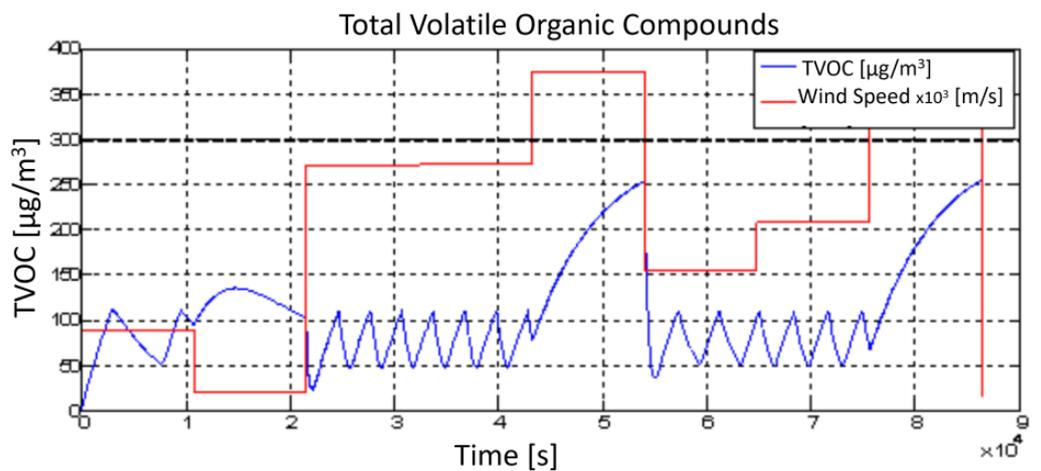
Figure 24. Control results: IAQ control, TVOC (CV).
