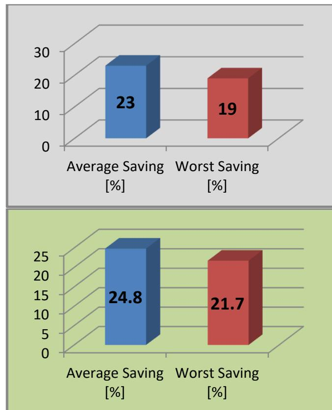
**Figure 42.** Energy saving results (average yearly energy savings and worst yearly energy savings): *initial* control system (**top**) and *modified* control system (**bottom**).
