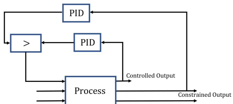
**Figure 2.** Override control architecture with high-pass selector logic [37].
