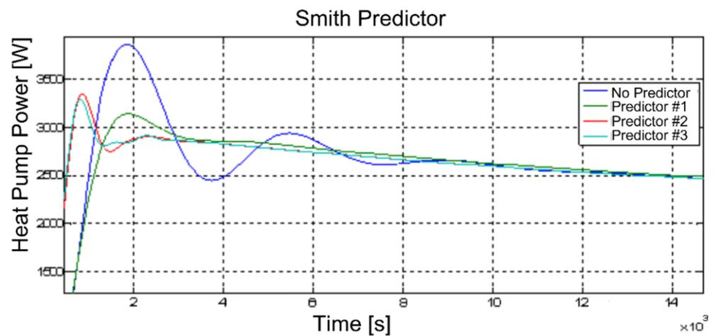
Figure 21. Control results: Smith predictor architecture performances (MV).
