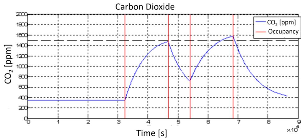
Figure 16. Modelization results on IAQ variables: CO<sub>2</sub>.
