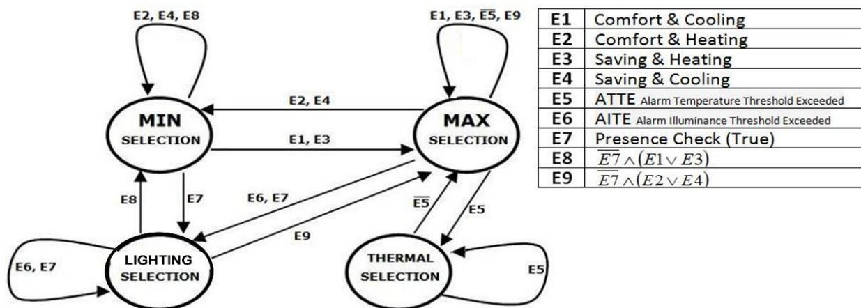
**Figure 12.** Personal comfort logic (PCL) module configuration (*modified* control system).
