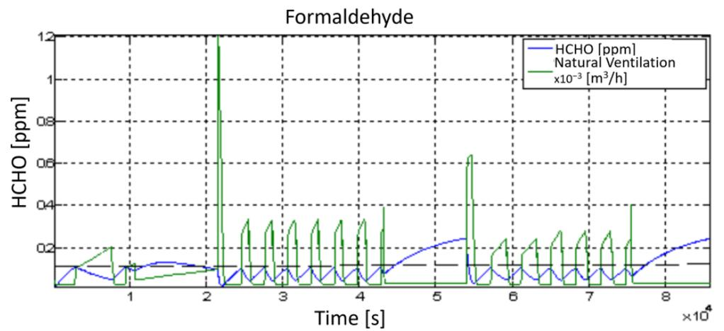
Figure 23. Control results: IAQ control, HCHO (CV).
