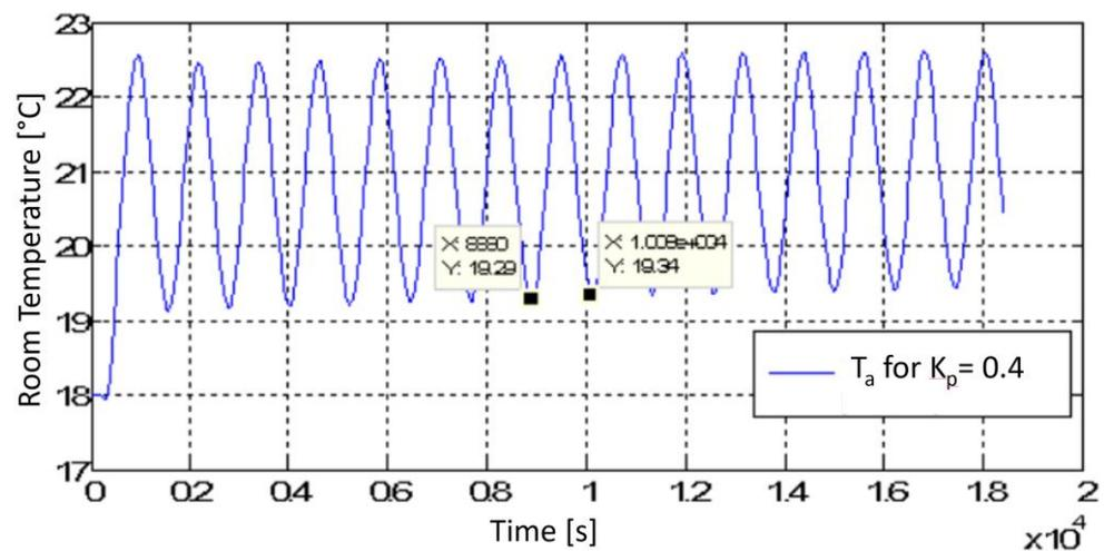
Figure 19. Control results: Smith predictor architecture tuning.
