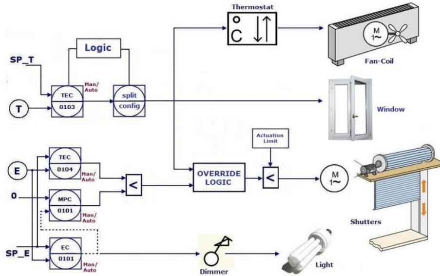
Figure 8. Architecture of the *initial* control system.
