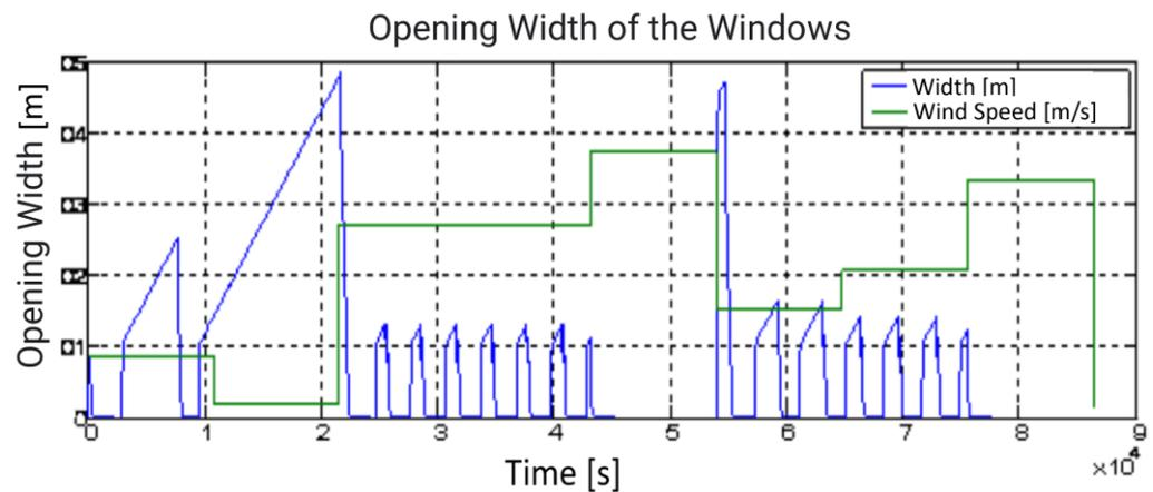
Figure 25. Control results: IAQ control, windows opening (MV).
