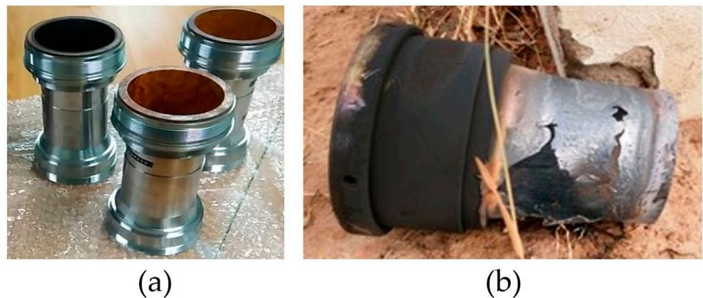
**Figure 1.** Samples of the 122 mm supersonic rocket nozzle (a) before and (b) after the mission, exhibiting excessive ablation.
