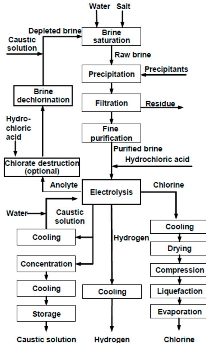
Figure 4. Process flow of simplified membrane cell process [26].
