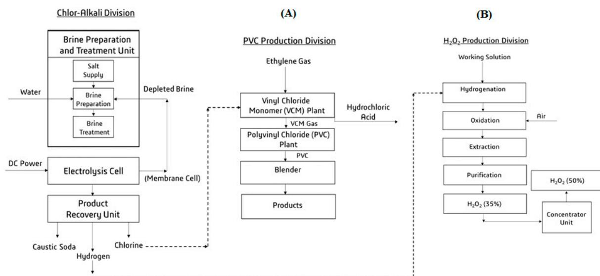
**Figure 7.** Combined Process Flow Diagram of Chlor-Alkali Process and PVC Processing Using Chlorine (A) and Integration of Chlor-Alkali Process and  $\text{H}_2\text{O}_2$  production Unit (B).
