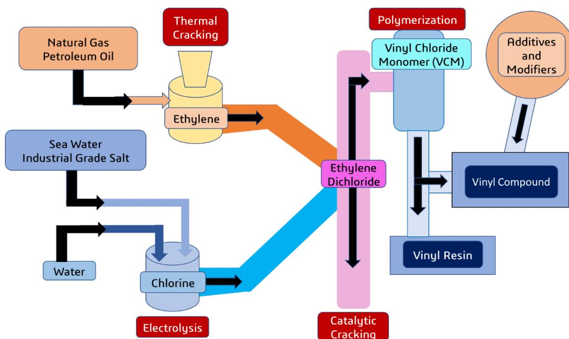
Figure 6. The generalized production process of vinyl resin [29].
