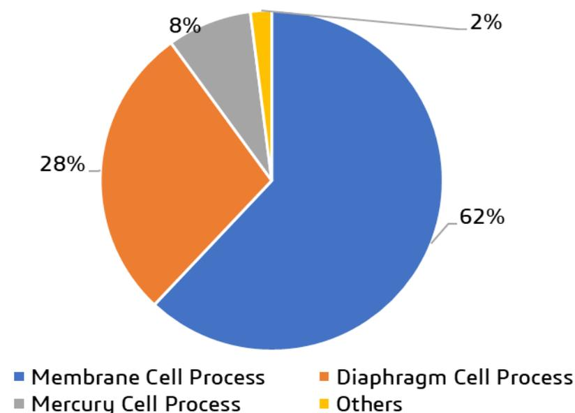
**Figure 3.** The division of capacity among the three principal cell technologies used in the world for chlor-alkali process [5].
