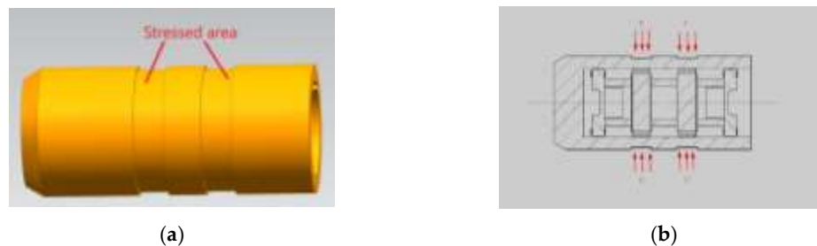
Figure 8. Assembly and stress diagram of piezomagnetic sensor. (a) Stress area diagram of sleeve, (b) Force diagram of sensor.
