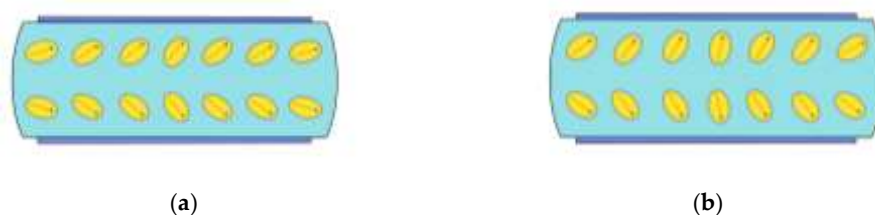
Figure 7. Variation diagram of magnetic domain under different magnetic induction intensity. (a) 105.35 kA/m. (b) 14.74 kA/m.
