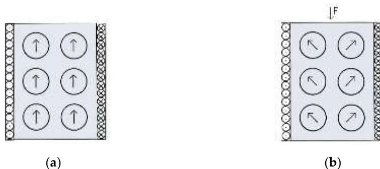
Figure 1. Magnetic domain distribution in iron-cobalt cylinder without force and under force. (a) Magnetic domain without force. (b) Magnetic domain under force.
