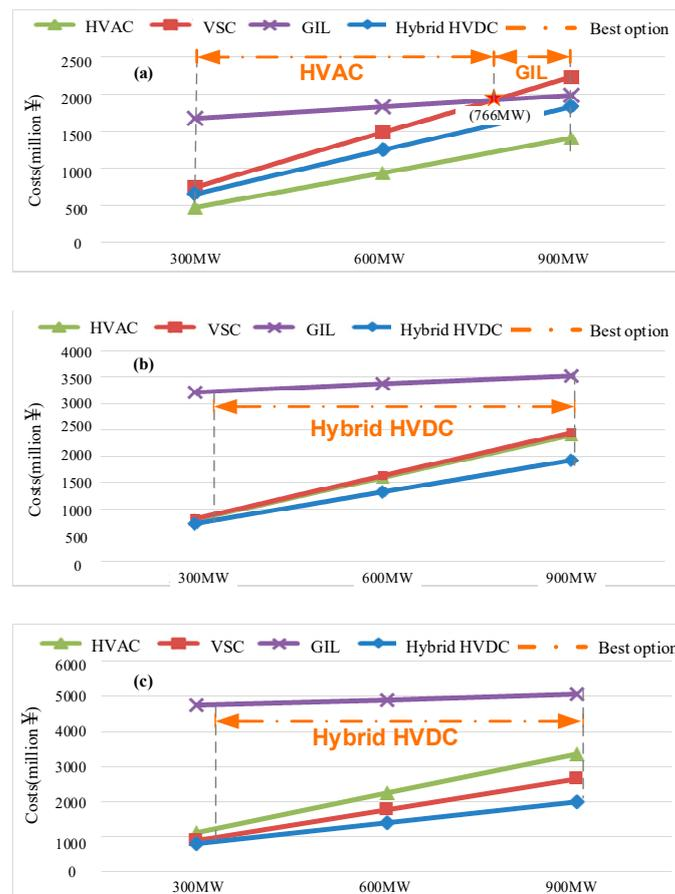
**Figure 5.** Total costs of different P of 25 km, 50 km, and 75 km wind farms: (a) shows the 25 km offshore wind farms total costs with different capacity; (b) shows the 50 km offshore wind farms total costs with different capacity; (c) shows the 75 km offshore wind farms total costs with different capacity.
