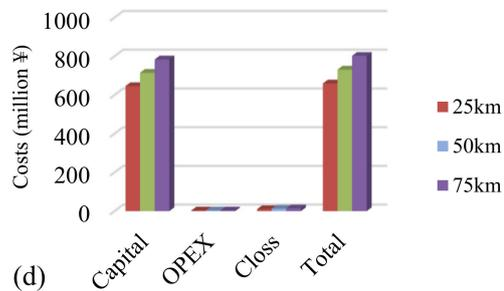
**Figure 4.** Cost component comparisons with different  $L$  ( $P$  is 300 MW): (a) shows the HVAC system; (b) shows the VSC-HVDC system; (c) shows the GIL system; (d) shows the Hybrid HVDC system.
