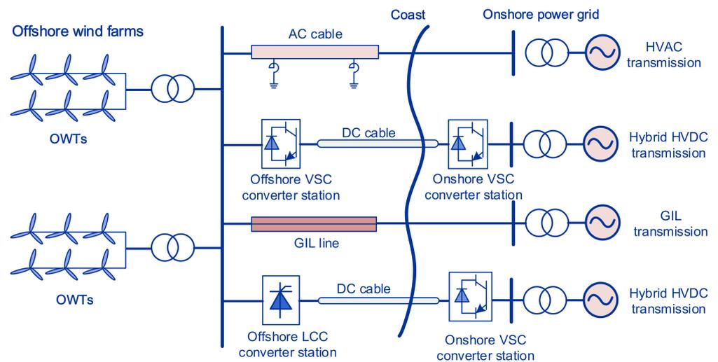
**Figure 2.** Structure of the four transmission methods for OWFs.
