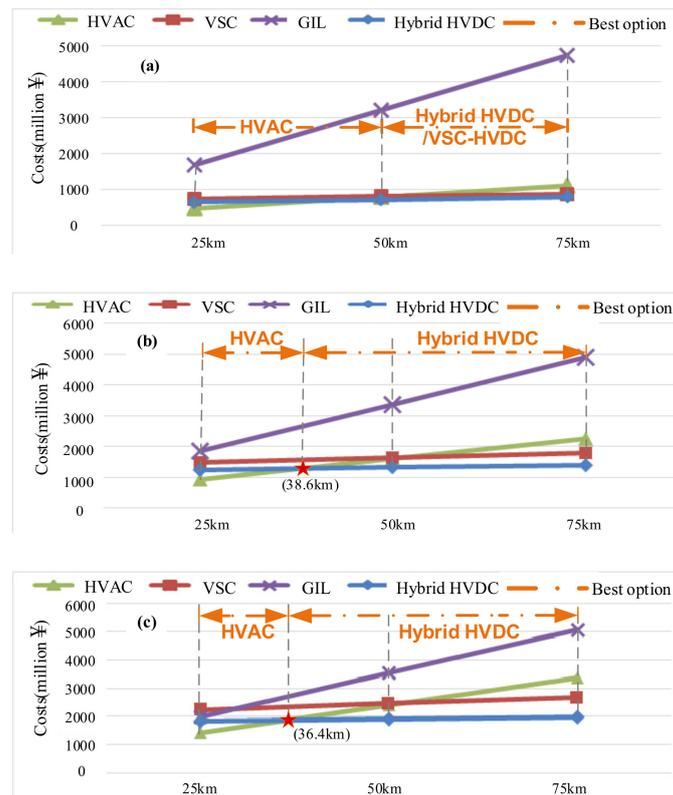
**Figure 3.** Total costs of different  $L$  of 300 MW, 600 MW, and 900 MW wind farms: (a) shows the 300 MW offshore wind farm total costs with different distances; (b) shows the 600 MW offshore wind farm total costs with different distances; (c) shows the 900 MW offshore wind farms total costs with different distances.
