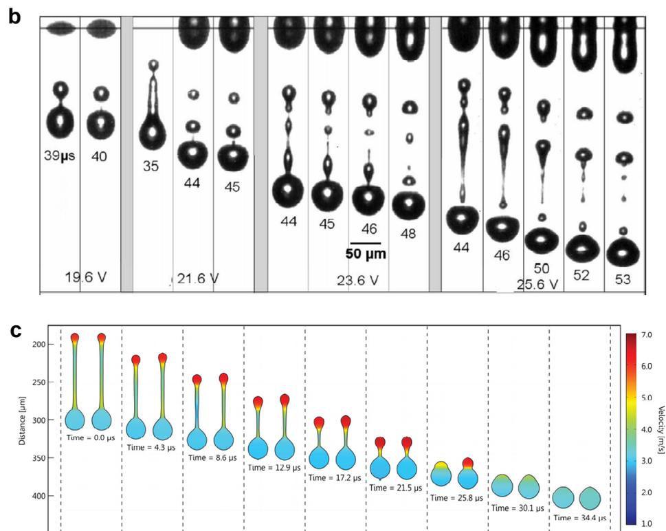
**Figure 2.** (a) Typical ink ejection, satellite formation, and recollection process (b) longer liquid thread will lead to the formation of multi-satellite droplets with a wide range of size and velocity; (c) retraction of the thread into one drop without breakup. Reproduced with permission from References [17,31].
