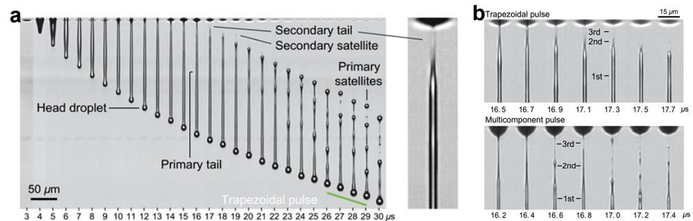
**Figure 4.** (a) Secondary tail formation during the ejection of viscous inks; (b) appearance of tertiary tails. Reproduced with permission from Reference [44].
