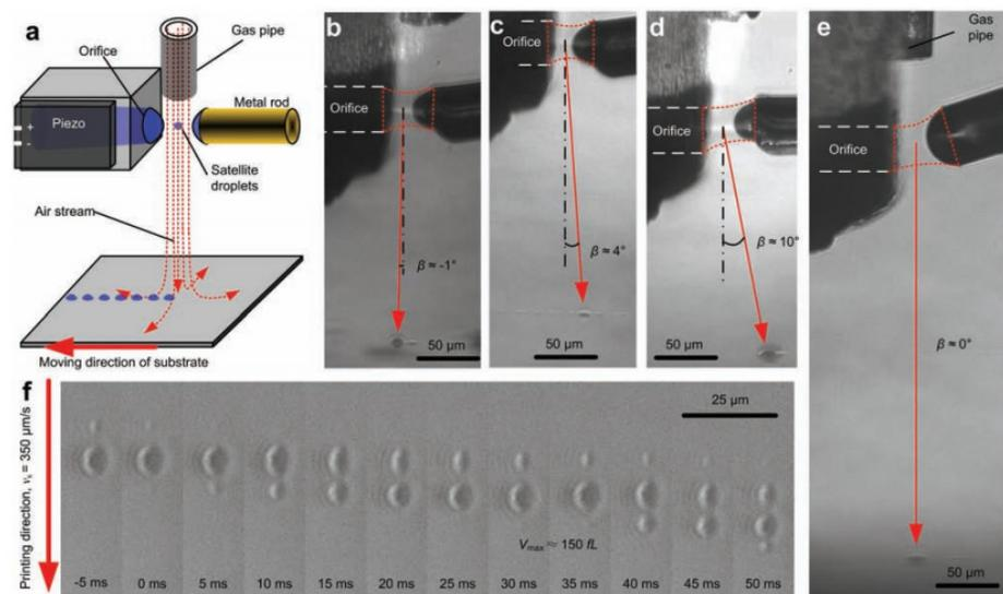
**Figure 8.** Illustration of satellite droplet printing. (a) Schematic setup; (b–e) images taken during printing with different settings; (f) drops printed on the glass. Reproduced with permission from Reference [86].
