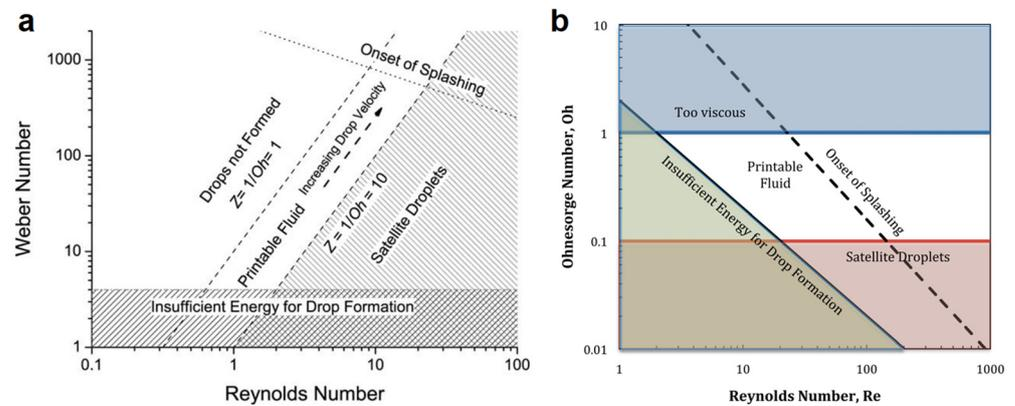
**Figure 1.** The operating regimes of inkjet printing in the control parameter space of (a) Weber number  $We$  versus Reynolds number  $Re$ , and (b) Ohnesorge number  $Oh$  versus Reynolds number  $Re$ . Reproduced with permission from References [25,30].
