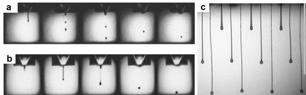
**Figure 6.** (a) Image sequence of drop formation for 50% glycerol/50% water created by a 50 V pulse with 79  $\mu$ s between each frame. (b) Image sequence of drop formation for a non-Newtonian solution (50 ppm of 300 k PEO in glycerol/water) created by a 50 V pulse amplitude with 79  $\mu$ s between frames. (c) A too-high polymer concentration leads to the formation of extremely long ligaments; The vertical scale bar (right) is 1 mm long. Reproduced with permission from References [75,79].
