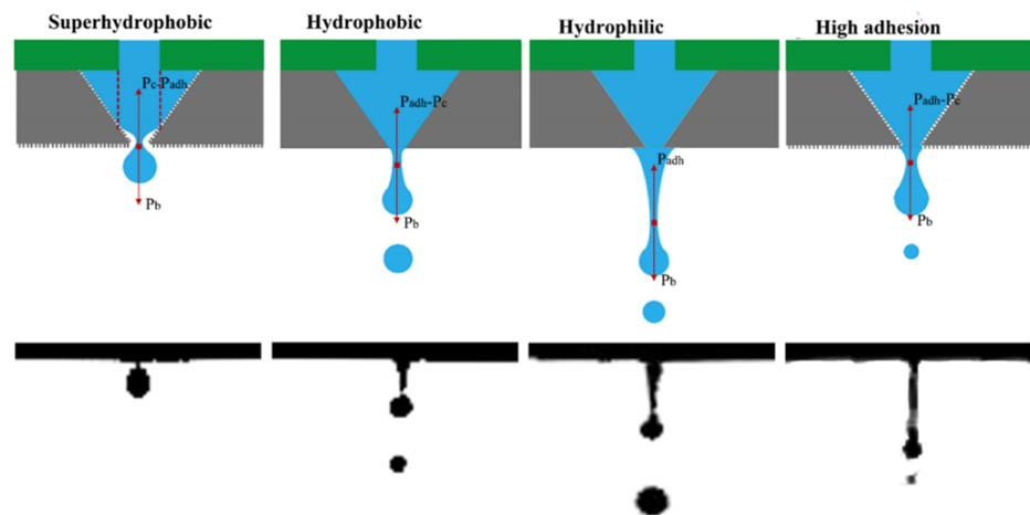
**Figure 7.** Mechanical analysis for the drop pinch-off and the corresponding experimental result for the superhydrophobic, hydrophobic, and hydrophilic nozzles and the superhydrophobic nozzle with high adhesion. Reproduced with permission from Reference [29].
