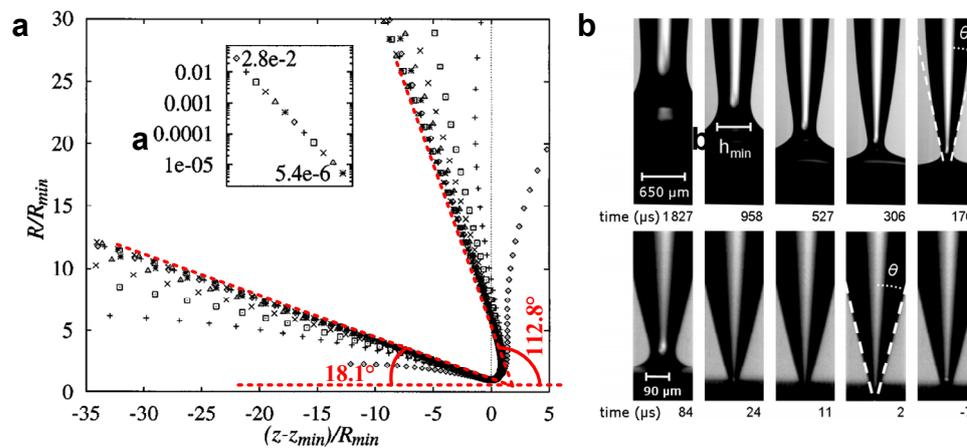
**Figure 3.** (a) The pinch-off shapes at various times collapse onto two cones when rescaled with minimum radius  $R_{min}(t)$  and centered on  $z_{min}(t)$ . (b) Imaging of the pinch-off region for a dripping water droplet shows a conge angle of about  $16.9^\circ$  (upper) and  $17.9^\circ$  (lower). Reproduced with permission from References [37,43].
