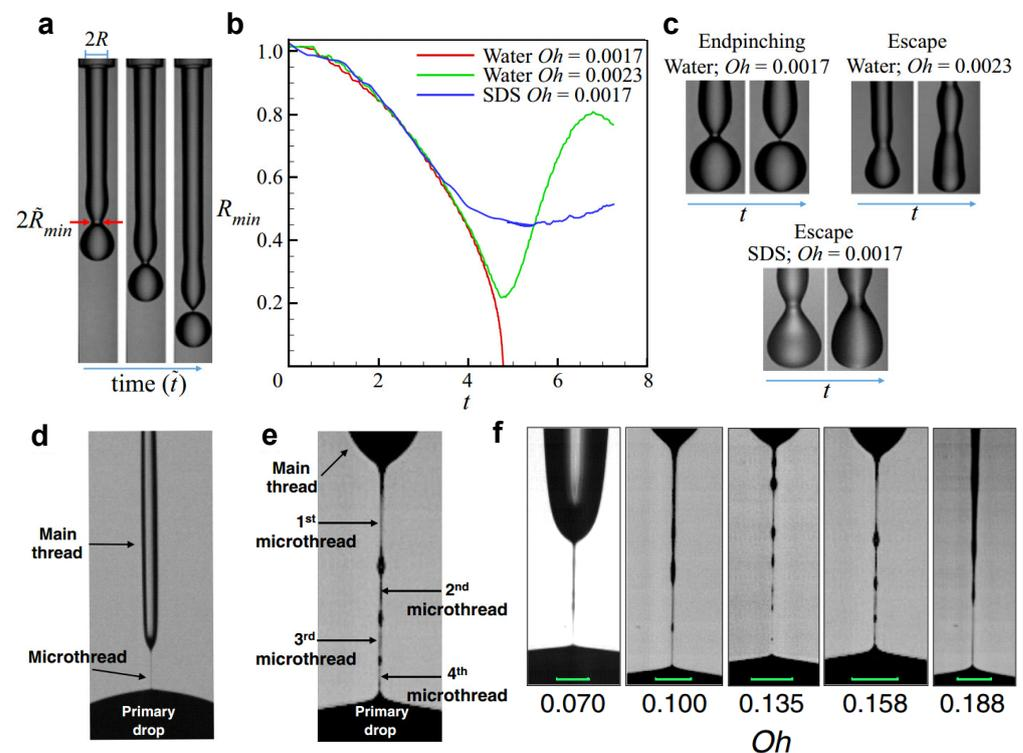
**Figure 5.** (a–c) An experiment carried out by Kamat et al. showed that end-pinching could be precluded in nearly inviscid filaments with the presence of surfactants by breaking up the process of the viscous glycerol-water thread (d) without and (e) with surfactant; (f) breakup shapes of glycerol-water thread loaded with sodium dodecyl sulfate (SDS) (concentration = 1.5 cmc) as a function of  $Oh$ . Reproduced with permission from References [66,68].
