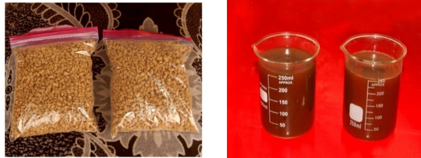
Figure 5. Pelletized solid and liquid digestates from rice husk.
