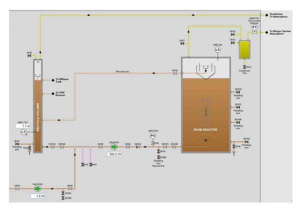
Figure 3. EGSB Reactor control and monitoring.
