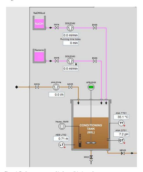
Figure 2. Feed wastewater control in the conditioning tank.
