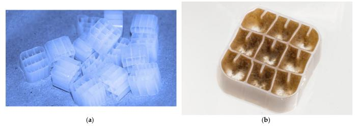
**Figure 4.** BWTX<sup>®</sup> carrier without biofilm growth (a) and with matured biofilm growth (b).
