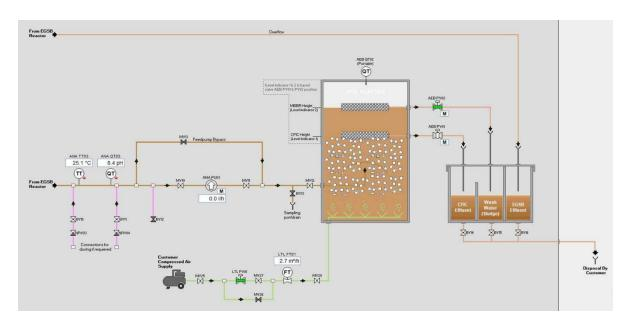
Figure 5. CFIC reactor control and effluent collection.
