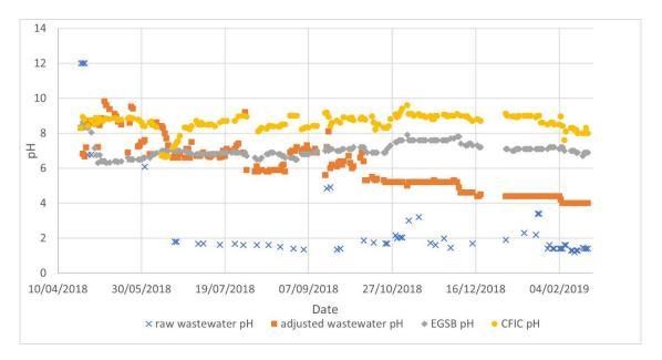
**Figure 6.** pH at different stages of the pilot study.
