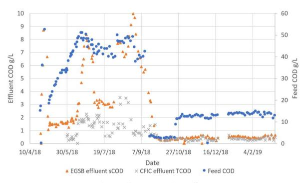
**Figure 7.** Feed, EGSB effluent sCOD and CFIC effluent TCOD concentrations.
