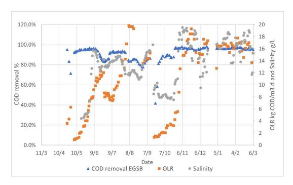
Figure 9. Relation of COD removal with salinity and organic loading rate.
