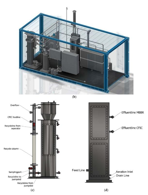
**Figure 1.** Drawings of the pilot units (a) Pilot units contents with wastewater and biogas flow direction marked; (b) overview of the 3D drawing. (c) EGSB unit layout. (d) CFIC reactor layout.
