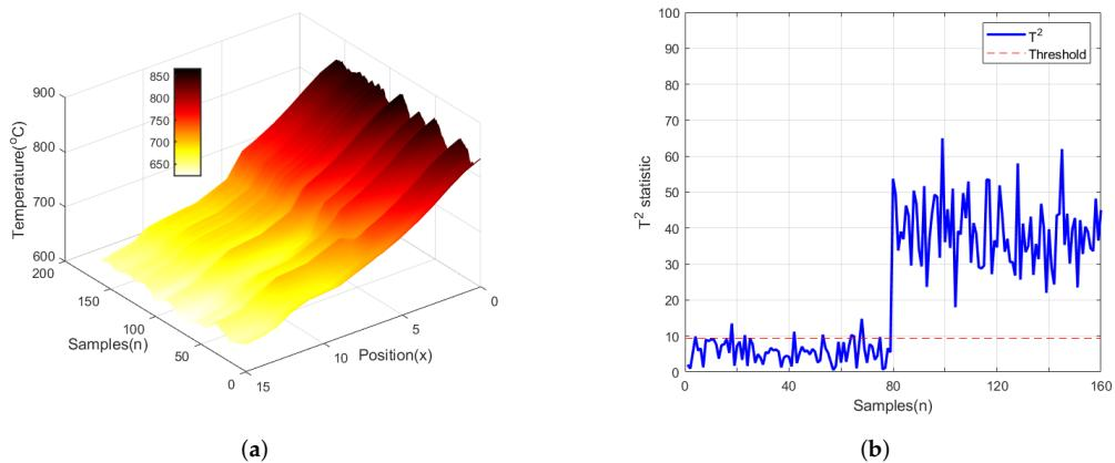
**Figure 13.** The temperature distribution (a) and monitoring result (b) of fault two.
