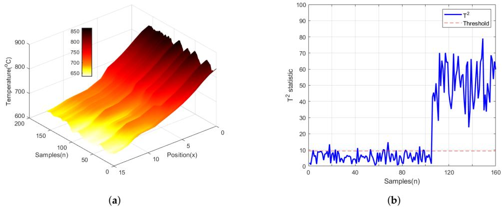
**Figure 12.** The temperature distribution (a) and monitoring result (b) of fault one.
