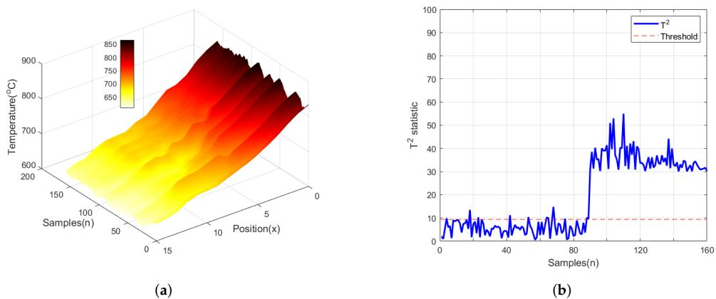
**Figure 14.** The temperature distribution (a) and monitoring result (b) of fault three.
