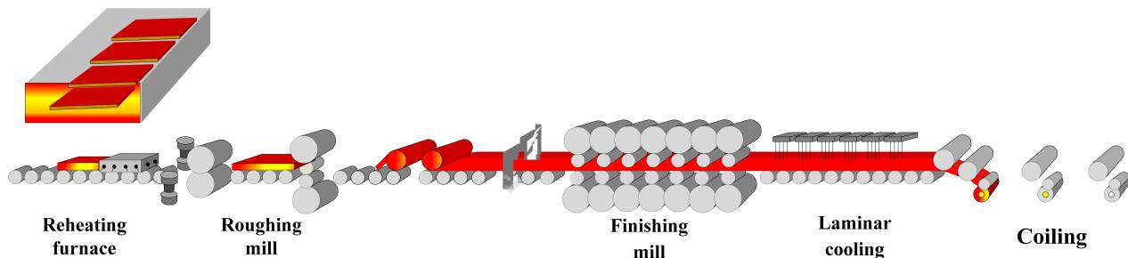
**Figure 1.** The flowchart schematic diagram of hot steel strip rolling.
