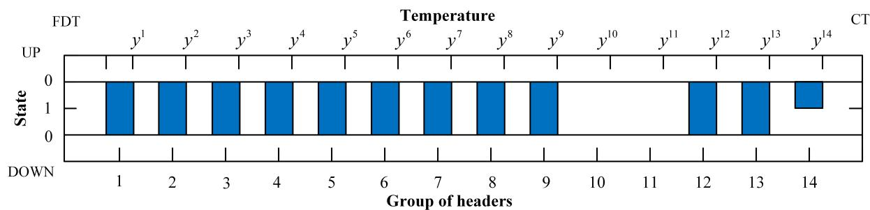
**Figure 7.** The initial state of spray header banks in LCP.
