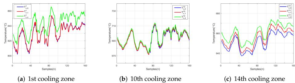
**Figure 9.** Spatial variation of the strip temperature in the 1st (a), the 10th (b), and the 14th (c) cooling zones.
