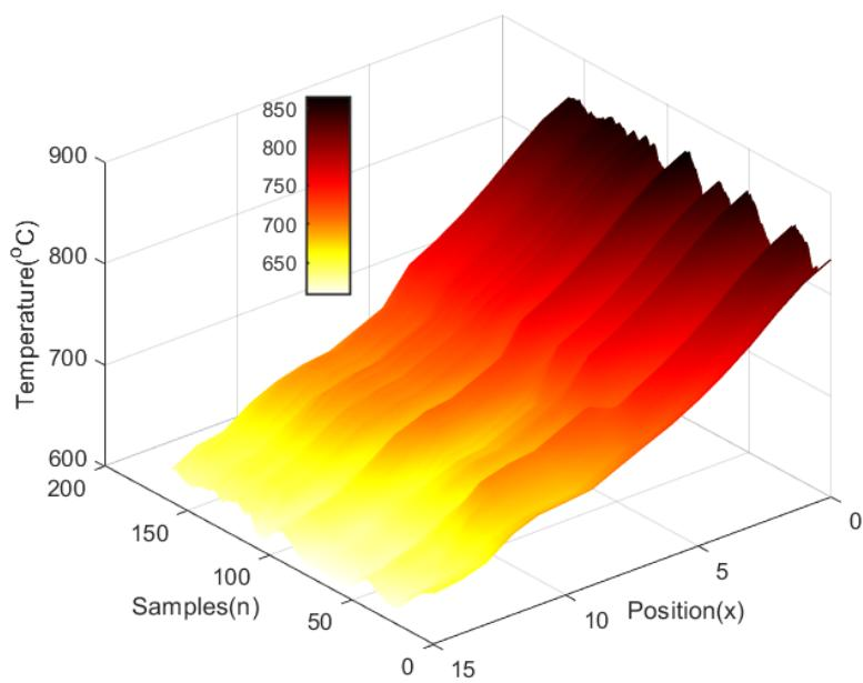
**Figure 10.** The spatial distribution of the strip temperature in normal condition.
