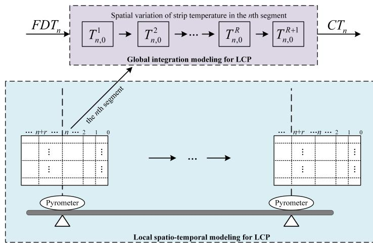
**Figure 5.** Time–space variation of the strip temperature for LCP.
