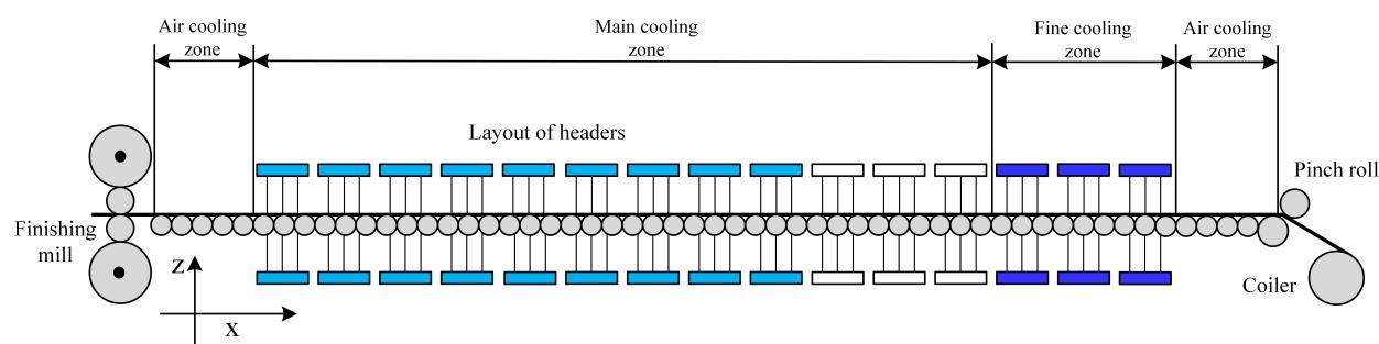
**Figure 2.** The schematic diagram of laminar cooling process.
