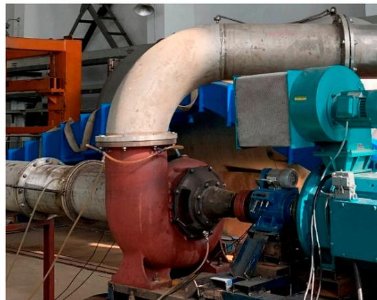
Figure 4. Test bench of a mixed-flow pump with a volute.
