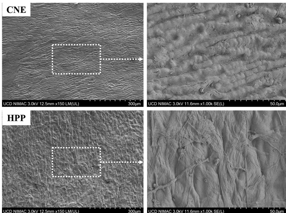
**Figure 6.** Scanning electron micrographs of the surface structure of Buckwheat hull before and after novel extraction at magnifications—300  $\mu\text{m}$  and 50  $\mu\text{m}$ .
