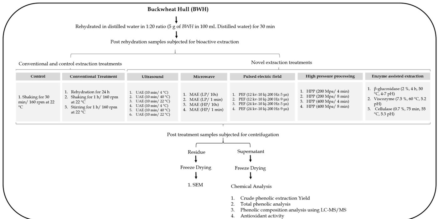
**Figure 1.** Schematic workflow of the bioactive extraction protocols employed to obtain phenolic extracts from buckwheat hull.
