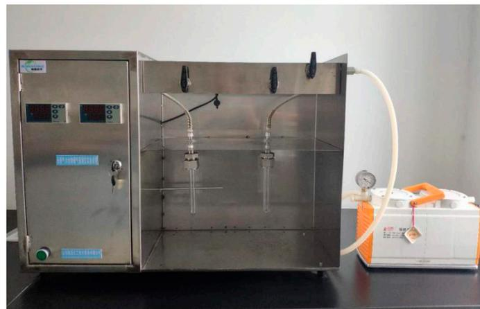
**Figure 3.** Gas storage capacity measurement device.
