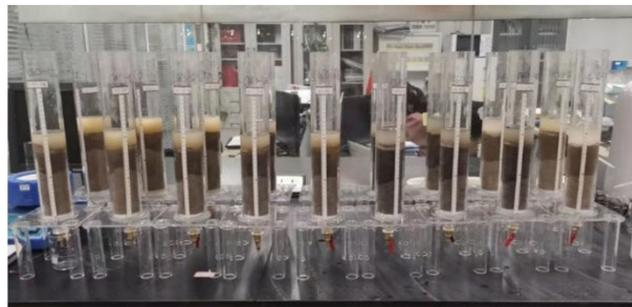
**Figure 9.** Soil column experiment.
