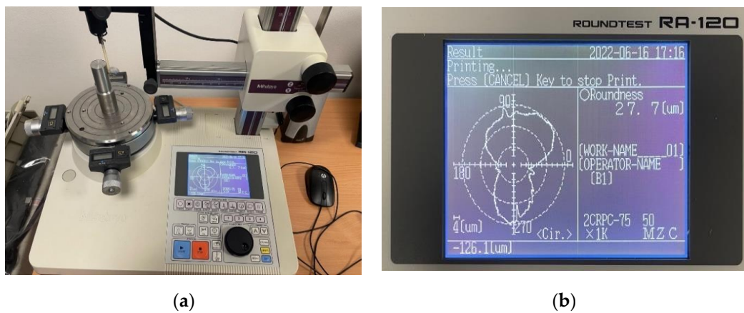
Figure 8. (a) Measurement of roundness deviation using the Roundtest RA-120; (b) device display with measured curve.
