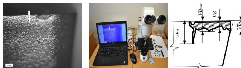
Figure 4. Analysis and measurement of the flank wear of the insert ( VB_N ) using a Carl Zeiss Primotech D/A ESD microscope (Zeiss Group, Oberkochen, Germany).
