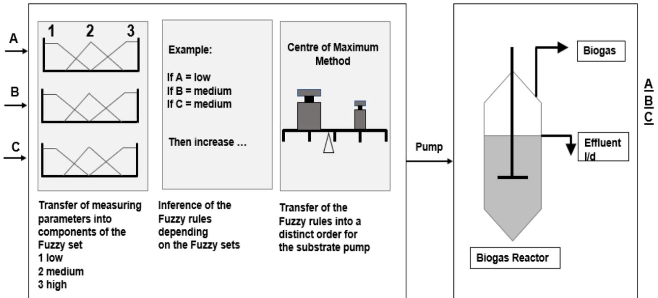
Figure 2. Scheme explaining the principle of the FLC system used for the performed biogas production process on a pilot-scale. A, B, and C are the three selected control parameters, representing the methane content (CH<sub>4</sub>), pH, and the specific GPR (spec. GPR).
