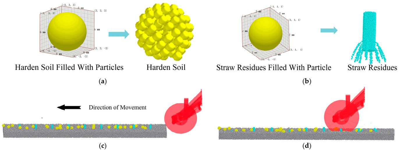
Figure 21. Simulation diagram of anti-sticky performance of seeding monomer digital twin. (a) Soil particle setting; (b) Maize particle setting; (c) Particle generation and equipment motion constraints added; (d) Simulation is running.
