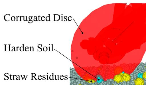
Figure 22. Schematic diagram of DT crushing simulation of corrugated disc. (a) Harden soil construction; (b) Straw residues construction; (c) Particle-bed construction and motion constraint added; (d) Running process of simulation.
