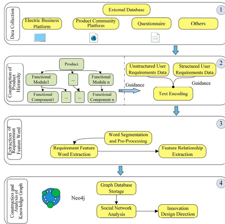
**Figure 4.** The process of constructing a user requirements knowledge graph.
