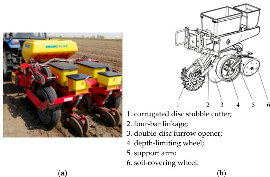
**Figure 12.** Schematic diagram of the seeding monomer of no-tillage maize planter. (a) Schematic diagram of the no-tillage maize planter; (b) Schematic diagram of the seeding monomer.
