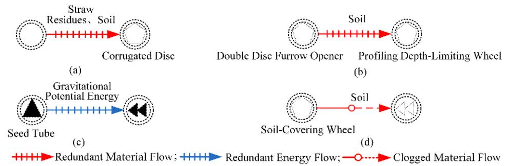
**Figure 16.** Simulation results of anti-sticky performance of seeding monomer digital twins. (a) Soil adhesion situation on corrugated disc; (b) Soil adhesion situation on profiling depth–limiting device; (c) Pressing situation on seed–pressing wheels; (d) Soil adhesion situation on soil–covering wheel.
