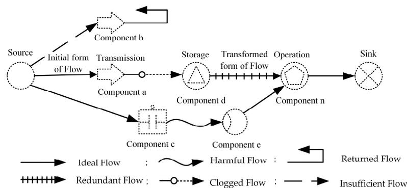
Figure 11. Signal flow function model in virtual domain.
