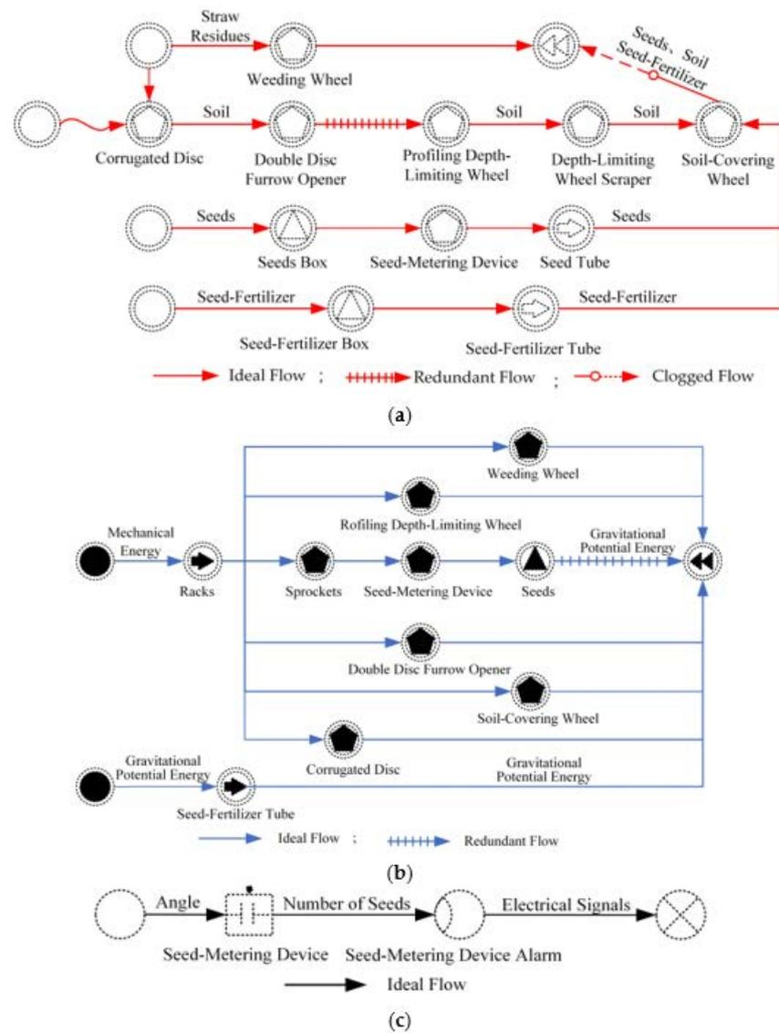
**Figure 15.** The flow function model of no-tillage seeding monomer. (a) Material flow function model; (b) Energy flow function model; (c) Signal flow function model.
