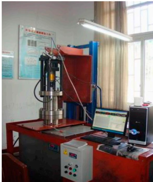
**Figure 2.** The triaxial servo-controlled seepage equipment for thermofluid–solid coupling of coal containing methane.
