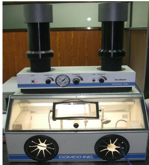
**Figure 2.** Micro-abrasive jet blaster.
