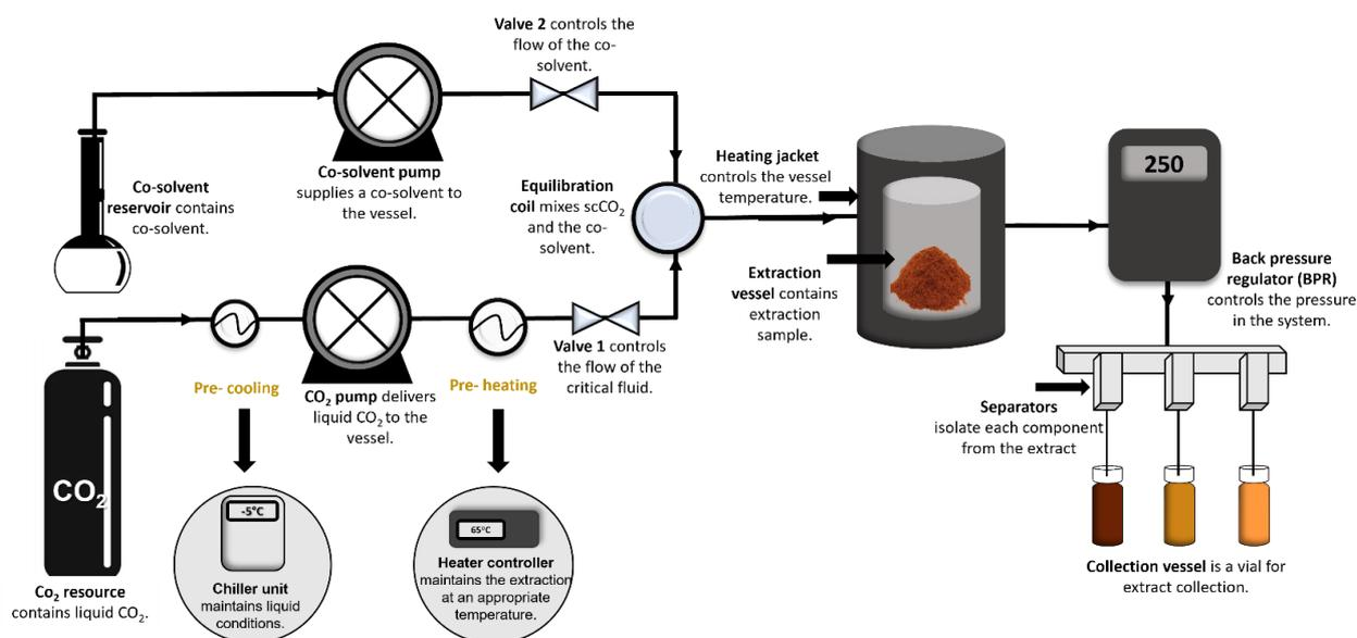
**Figure 4.** Schematic of the laboratory-scale supercritical fluid extractor.
