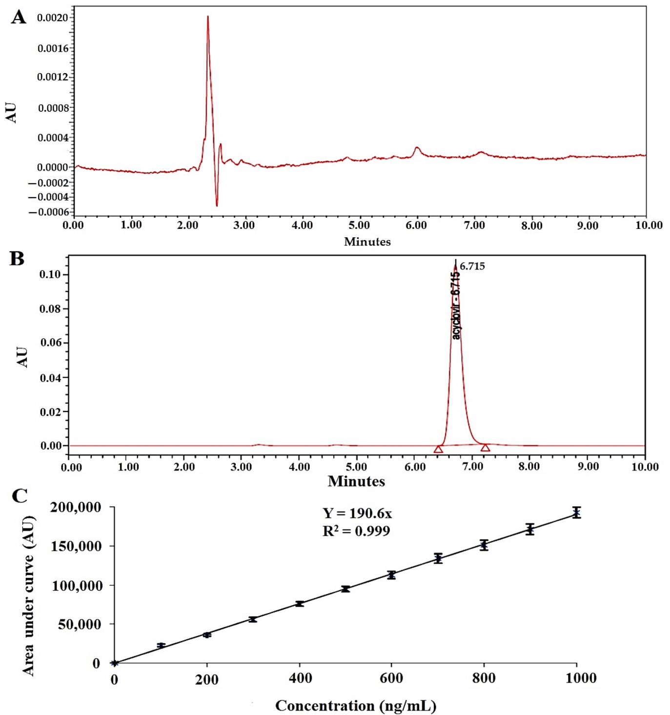
Figure 4. (A) Blank plasma, (B) chromatogram of ACV in plasma, and (C) calibration plot of ACV in plasma.
