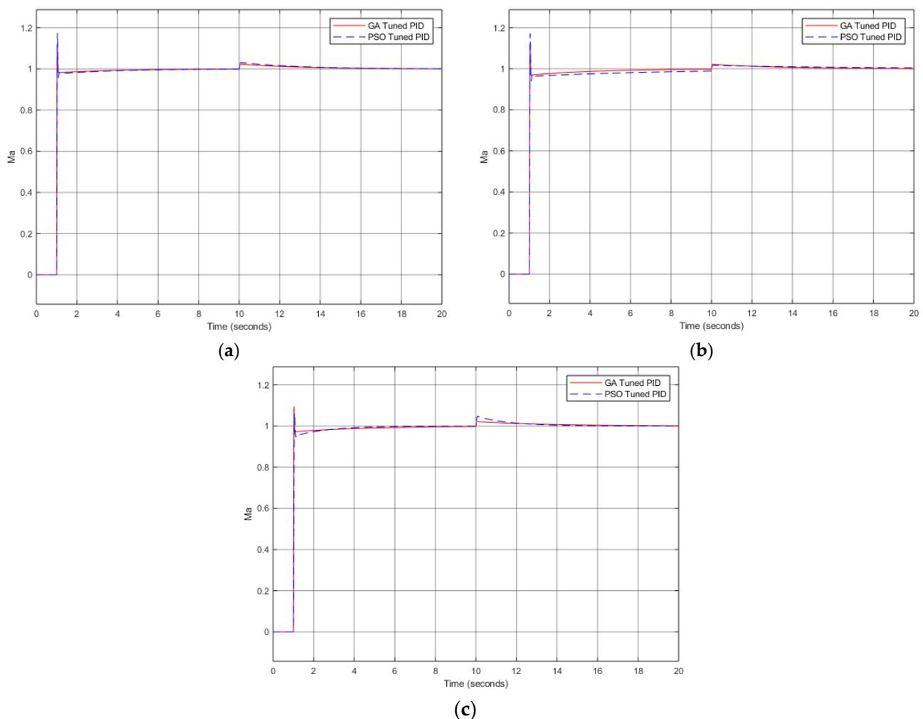
**Figure 4.** Mach number control results. (a) Mach 0.6. (b) Mach 0.8. (c) Mach 1.0.
