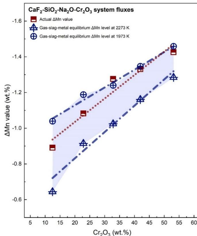
**Figure 6.** Actual and predicted  $\Delta\text{Mn}$  levels as a function of the  $\text{Cr}_2\text{O}_3$  addition level in the flux.
