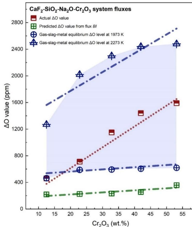
**Figure 2.** Actual and predicted  $\Delta O$  levels as a function of the  $Cr_2O_3$  addition level in the flux.
