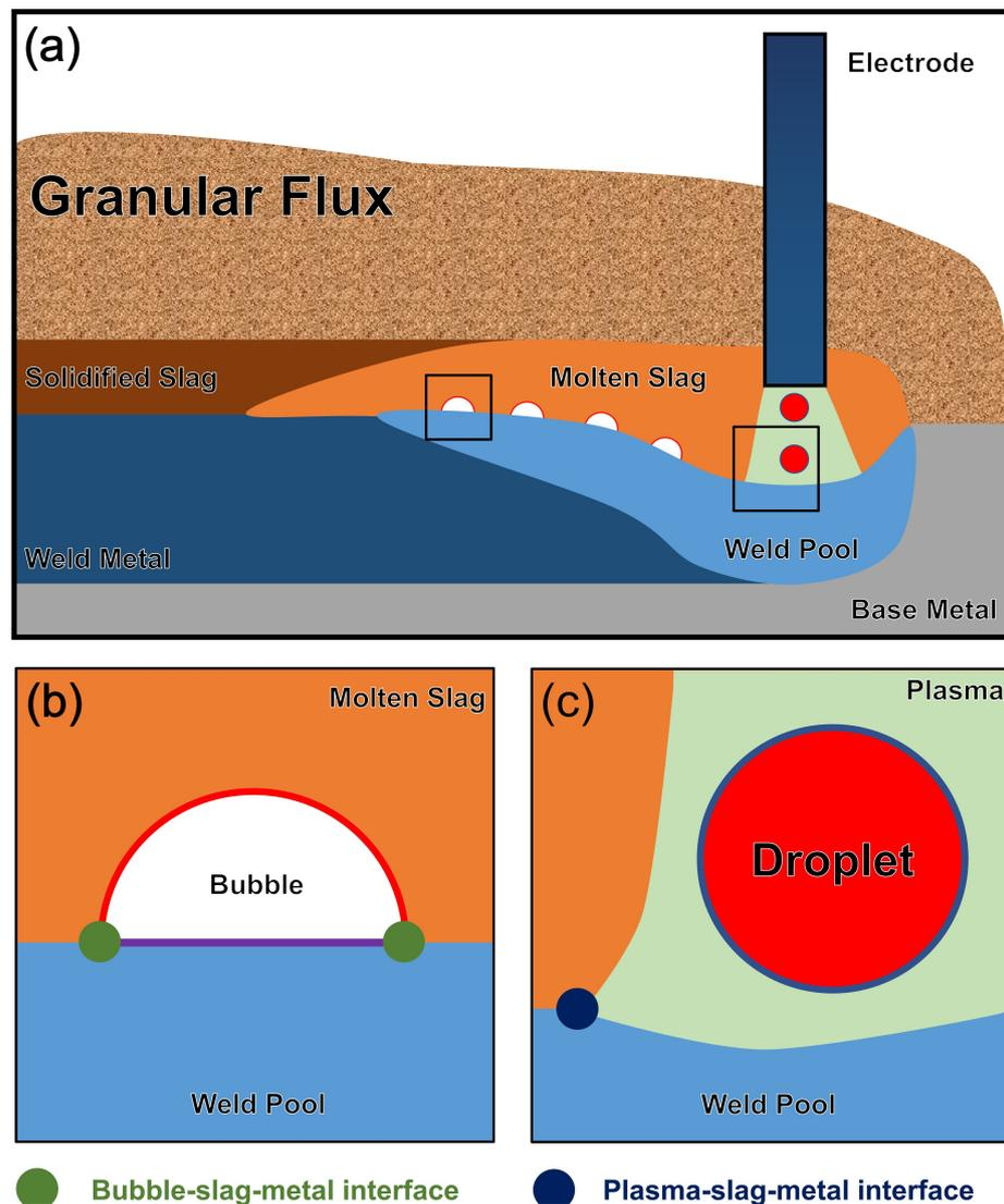
**Figure 1.** Major phases and reaction interfaces associated with gas phases in SAW: (a) Schematic diagram of SAW, (b) Plasma-associated reaction interfaces, (c) Bubble-associated reaction interfaces.
