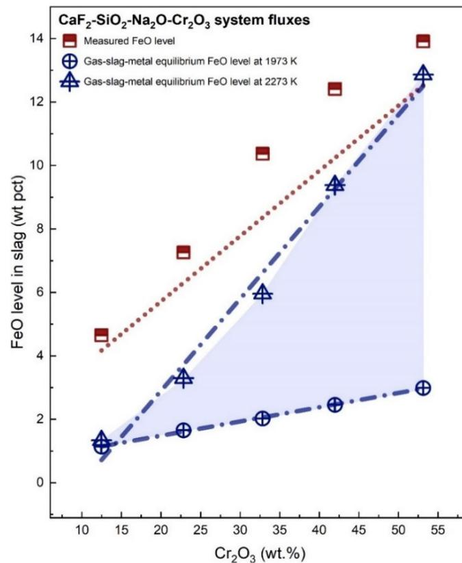
**Figure 3.** FeO level in the slag as a function of the  $\text{Cr}_2\text{O}_3$  addition level in the flux.
