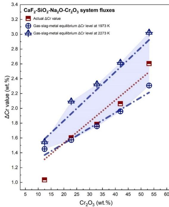
**Figure 4.** Actual and predicted  $\Delta\text{Cr}$  levels as a function of the  $\text{Cr}_2\text{O}_3$  addition level in the flux.
