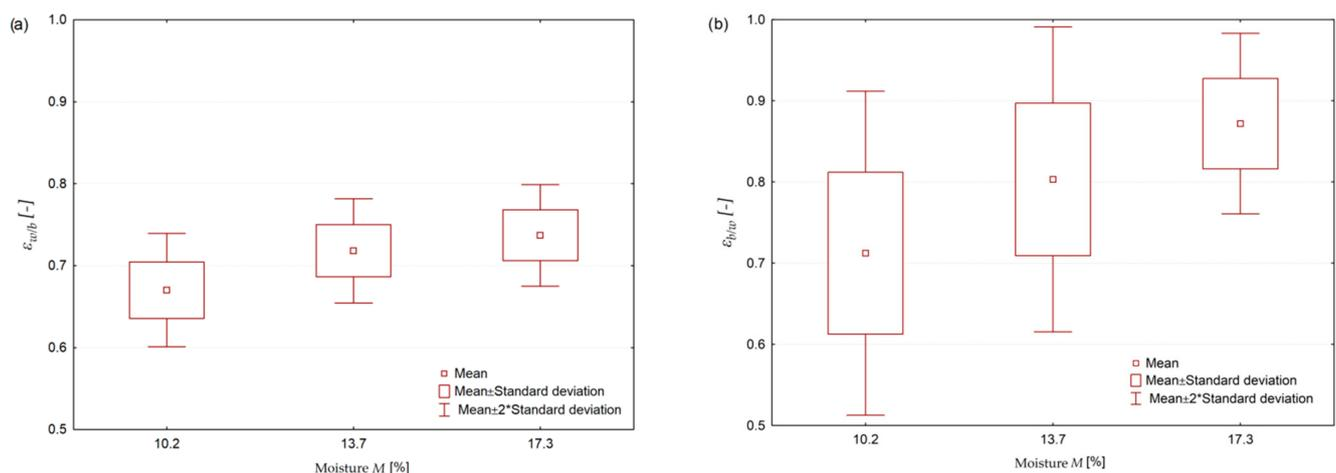
**Figure 4.** Mean values of separation efficiency  $\epsilon$ , subject to the moisture  $M$  content of mixture components: (a)—mixture of wheat kernels and buckwheat nutlets ( $\epsilon_{w/b}$ ); (b)—mixture of buckwheat nutlets and wheat kernels ( $\epsilon_{b/w}$ ).
