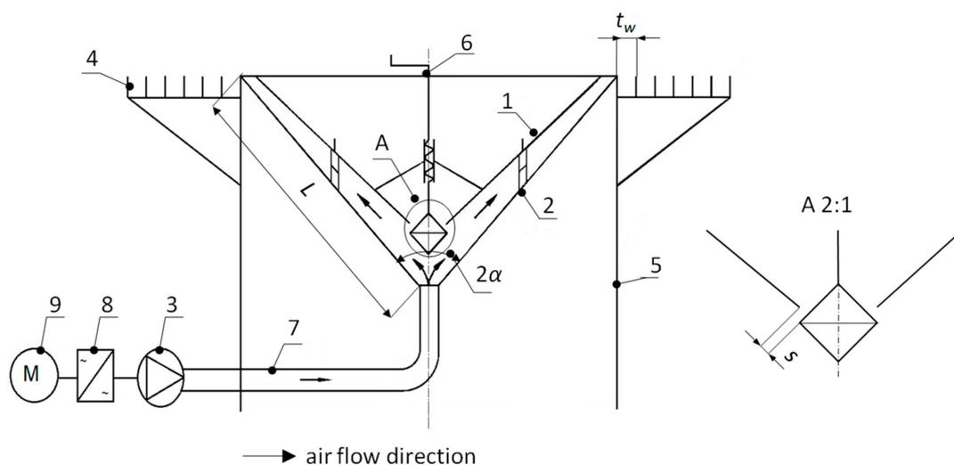
**Figure 2.** Diagram of the test stand: 1—inner cone working surface, 2—outer cone surface, 3—fan, 4—troughs, 5—base, 6—knob for infinitely variable adjustment of the charging slot, 7—air duct, 8—power inverter, 9—electric motor,  $2\alpha$ —cone's apex angle,  $L$ —length of the cone's generating line,  $s$ —width of the grain inlet,  $t_w$ —through width.
