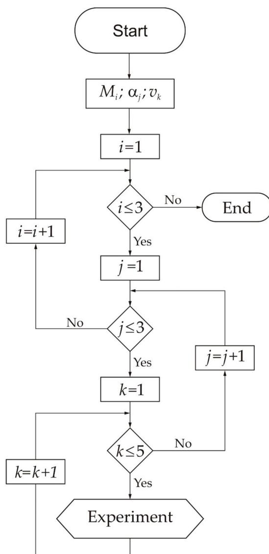
**Figure 3.** Algorithm for separating the seed mixture in a pneumatic conical separator:  $i, j, k$ —values of variable parameters ( $M, \alpha, v$ ).
