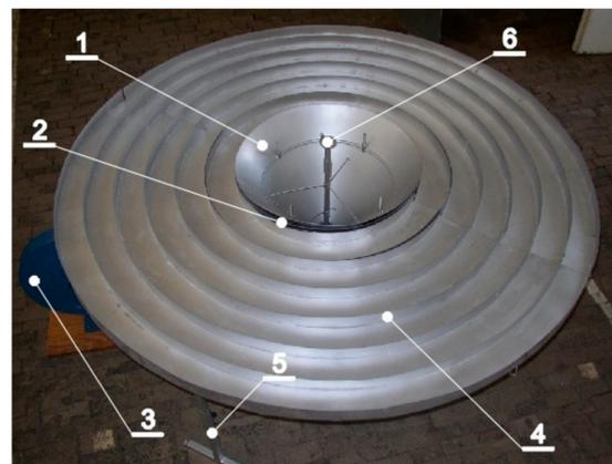
**Figure 1.** Test stand: 1—inner cone surface, 2—outer cone surface, 3—fan, 4—troughs, 5—base, 6—knob for infinitely variable adjustment of the charging slot.
