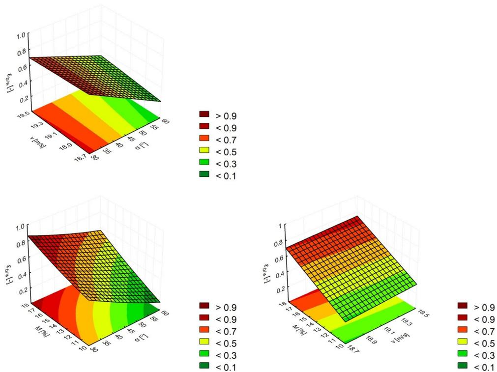
**Figure 6.** Separation efficiency index of the mixture of buckwheat nutlets and wheat kernels ( $\epsilon_{b/w}$ ) for seeds with different moisture content ( $M$ ), separated at different air stream velocities ( $v$ ), and different cone apex angles ( $\alpha$ ).
