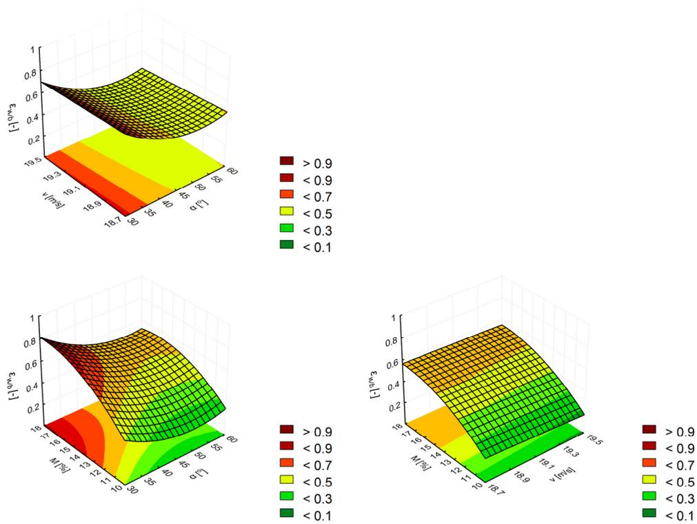
**Figure 5.** Separation efficiency index of the mixture of wheat kernels and buckwheat nutlets ( $\epsilon_{w/b}$ ) for seeds with different moisture content ( $M$ ), separated at different air stream velocities ( $v$ ), and different cone apex angles ( $\alpha$ ).
