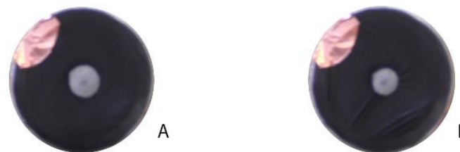
Figure 2. Inverted graphite dielectric elastomer actuator (DEA) silicone membrane tested in this study: (A) deactivated DEA (12 mm); (B) activated DEA (5 mm).
