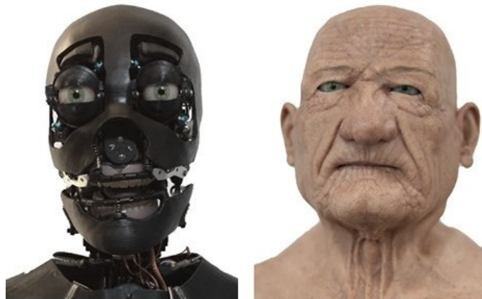
Figure 12. Realistic Humanoid Robot Euclid with non-dilating acrylic Eyes. Left: exoskeleton. Right: RHR with skin.
