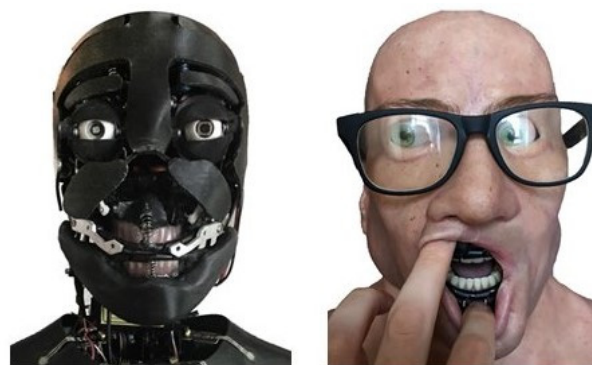
Figure 9. Robotic eye installation in RHR ‘Baudi’ for testing. Left: Exoskeleton. Right: Finished robot with skin and gelatin eye membranes.
