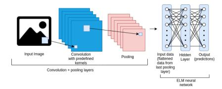
**Figure 6.** Example of a CELM architecture composed of a CNN with pre-defined kernels for feature extraction and an ELM for fast learning. The convolution and pooling layers' quantities can be varied. Also, the kernels pre-defined in the convolution layers can be based on different distributions. At the end of the feature extraction process, an ELM network makes the learning process.
