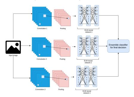
**Figure 7.** Example of ensemble representation for CELM. Three different CELM architectures are used for feature extraction and learning process. At the end, an operator is responsible for making the final classification decision.
