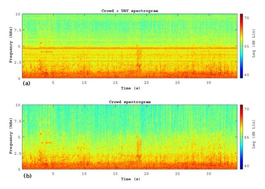
**Figure 5.** Spectrograms of two scenarios. (**a**) Noise produced by the crowd in the presence of a UAV in operation; (**b**) noise produced by the crowd. The samples refer to about 30 s of recording. To highlight the characteristic frequencies of the event, we have restricted the frequency range on the ordinate to the range 0–10 kHz. Recording in the presence of the UAV was performed by placing the UAV on the tripod at about 15 m from the registration station, as shown in Figure 1.
