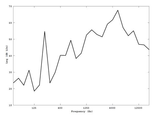
**Figure 3.** Average spectral levels in the one-third octave band between 50 Hz and 20 kHz (dB Lin) measured in the anechoic chamber. To simulate the flight conditions inside this limited volume chamber, the UAV was anchored to a tripod. In this configuration, several measurement sessions were carried out, bringing the UAV to maximum speed conditions. The measurements were performed with a Class 1 Solo 01-dB sound level meter, in accordance with the UNI EN ISO 3745:2012 standard [31].
