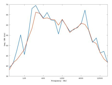
**Figure 4.** Average spectral levels in one-third octave band between 50 Hz and 12,500 Hz (dB Lin). The red curve represents the average spectral levels of the scenario with the crowd, while the blue curve represents the average spectral levels of the scenario with the crowd and the UAV.
