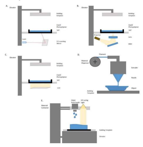
**Figure 2.** Three-dimensional printing technologies. (**A**) Laser-SLA, (**B**) DLP, (**C**) LCD, (**D**) FFF, and (**E**) PPP.
