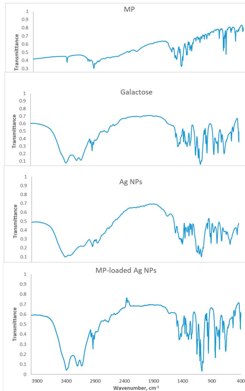
**Figure 3.** IR spectra of MP, galactose, galactose-assisted Ag NPs, and MP-loaded Ag NPs in the region 4000–400  $\text{cm}^{-1}$ .
