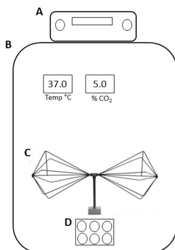
**Figure 1.** Schematic representation of the EMF exposure system. (A) Signal generator, (B) incubator, (C) biconical transmitting antenna, and (D) 6-well plate.
