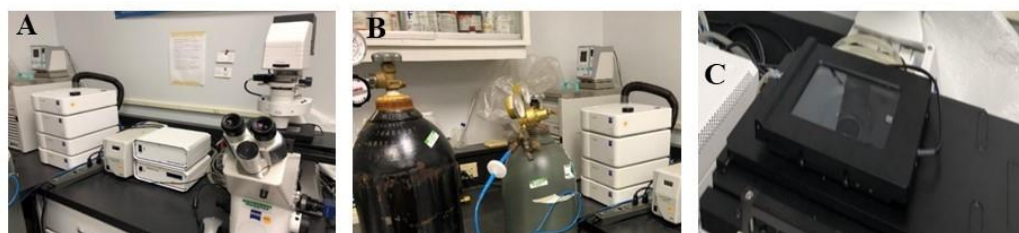
Figure 3. A complete fluorescent microscope setup is shown. (A) Set-up of the Zeiss Axio observer Z1 epifluorescent microscope, (B) 100% CO 2 and N 2 gas tanks and mixing modules and, (C) incubation chamber.
