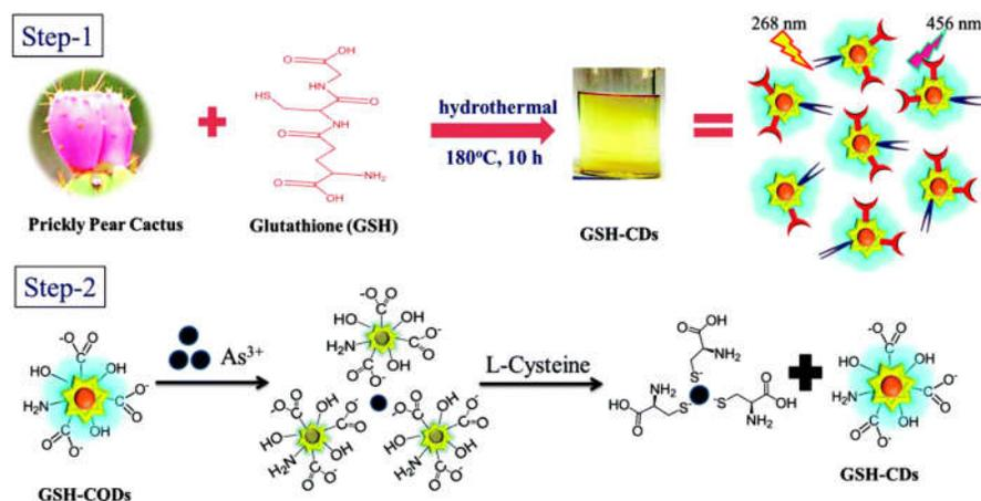
**Figure 5.** Illustration of synthetic route for obtaining GSH-CQDs and working principle toward the sensitive detection of As<sup>3+</sup> metal ions [120].
