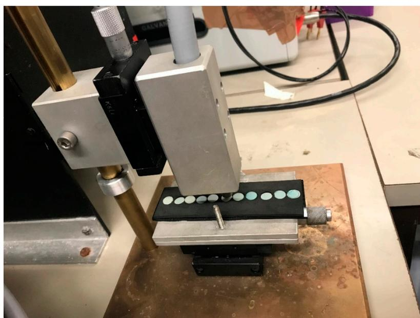
Figure S8. Close-up view on the dipsticks on the sample holder during detection.
