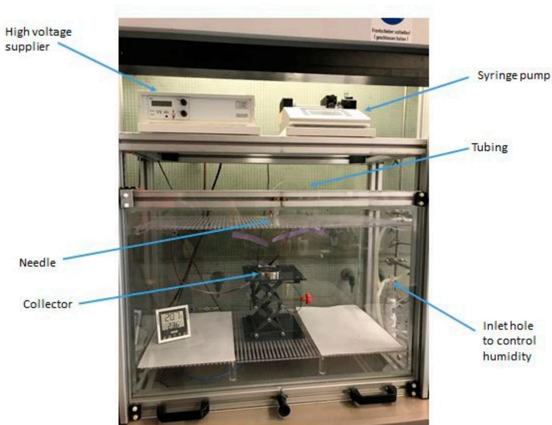
**Figure S1.** Image of the electrospinning setup with voltage supply and syringe pump.
