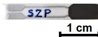
Figure 8. The thin nanocomposite layer after drop casting and drying on the sensor support with IDEs.
