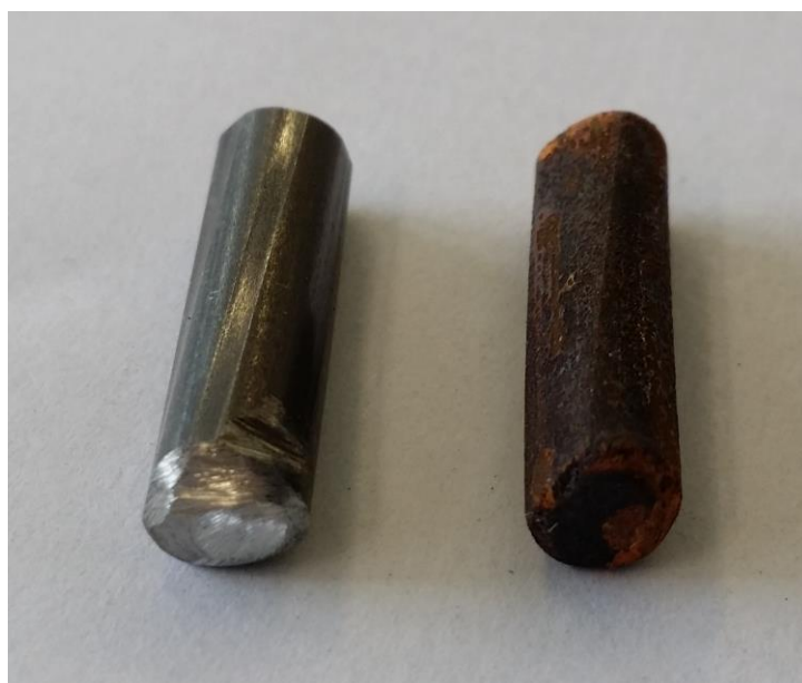
Figure 3. (Left) Blank uncorroded iron bar. (Right) Iron bar stored for three months outside with changing temperature and humidity initiating the corrosion process.
