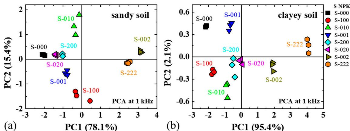
**Figure 4.** Principal component analysis (PCA) for the 1 kHz capacitance results of the e-tongue system applied to liquid aliquots of (a) sandy and (b) clayey soil samples enriched with different amounts of N, P and K.
