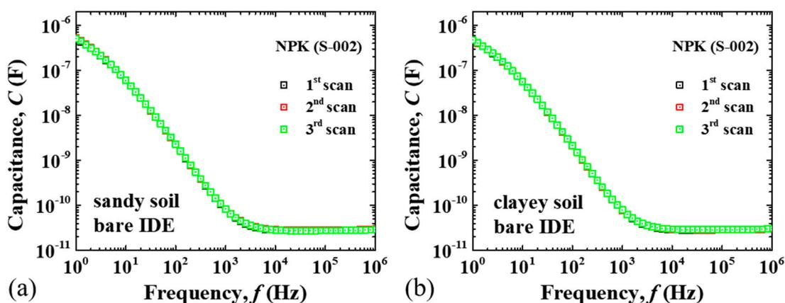
**Figure 3.** Capacitance versus frequency spectra measured with bare IDE sensing unit for (a) sandy and (b) clayey soil samples enriched with a higher amount of potassium (S-002) in aqueous solution at  $1 \text{ mg}\cdot\text{mL}^{-1}$ .
