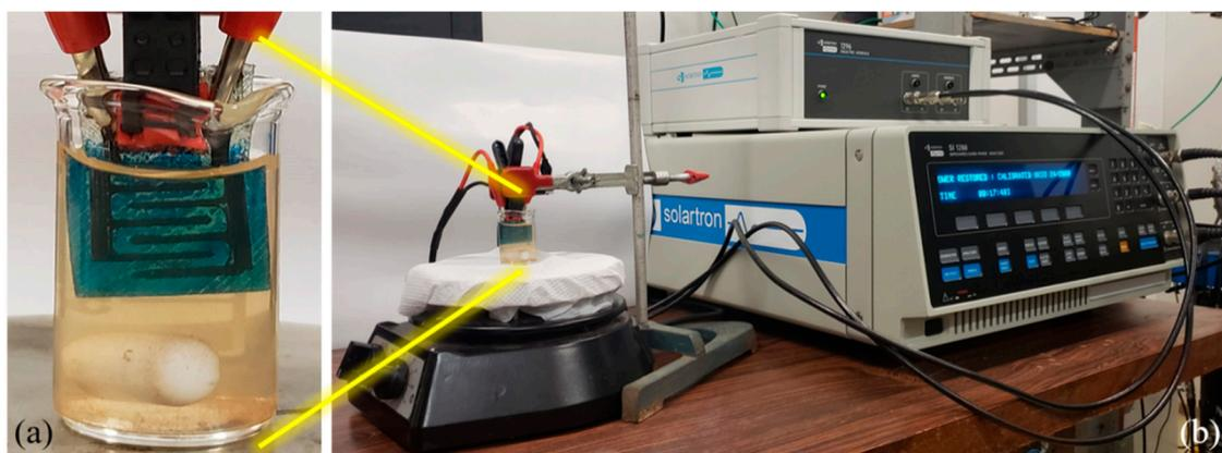
**Figure 1.** (a) Zoom at one of the sensing units (poly(diallyldimethylammonium chloride) solution/copper phthalocyanine-3,4',4'',4'''-tetrasulfonic acid tetrasodium salt (PDDA/CuTsPc)) in the beaker with a soil sample in aqueous solution and (b) experimental setup used for the e-tongue analysis with electrical measurements.
