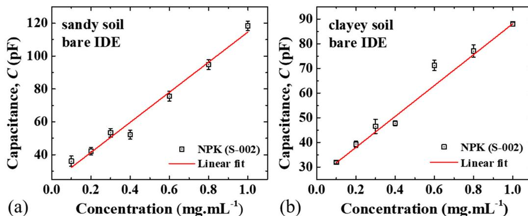
**Figure 5.** Capacitance data obtained for the bare IDE sensing unit at 1 kHz from 0.1 to 1 mg·mL<sup>-1</sup> of (a) sandy and (b) clayey soil samples enriched with a higher amount of potassium (S-002).
