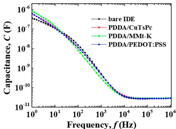
**Figure 2.** Capacitance spectra for the bare interdigitated electrodes (IDE), PDDA/CuTsPc, PDDA/montmorillonite clay (MMt-K), and PDDA/poly(3,4-ethylenedioxythiophene)-poly(styrenesulfonate) (PEDOT:PSS) sensing units in distilled water.
