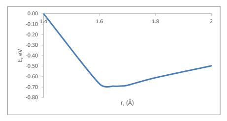
Figure 2. The CNT and an amino group interaction energy curve.
