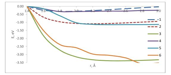
**Figure 3.** Energy curves of interaction between an amino-group modified nanotube with atoms and ions: 1 Li atom; 2 K atom; 3 Na atom; 4 Li<sup>+</sup> ion; 5 Na<sup>+</sup> ion; 6 K<sup>+</sup> ion, dependent on the distance between atoms/ions of metals and the hydrogen atom of the group.
