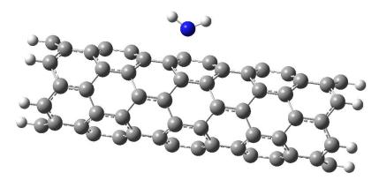
Figure 1. The CNT model with a surface functionalized by an amino group.
