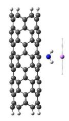
**Figure 4.** A scan of an arbitrary site on the surface modified carbon nanotube (6,0) that contain a Li atom (a pink color ball of a larger size); the dotted line indicates the route of Li atom movement in relation to an amino group functionally modified nanotube.
