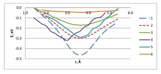
**Figure 5.** Energy curves of the scanning process of an arbitrary surface containing with atoms and ions: 1 Li atom; 2 K atom; 3 Na atom; 4 Li<sup>+</sup> ion; 5 Na<sup>+</sup> ion; 6 K<sup>+</sup> ion, surface-modified system "CNT +  $NH_2$ " The 1 Å point is located under the hydrogen atom of the amino group, to which the metal atom moves.
