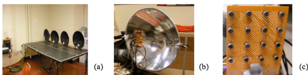
Figure 3. Two types of acoustic beam array that replace a single microphone element for improving PA sensing system: (a) An array of 4 microphones-reflector pairs; (b) One reflector with 16 microphones; (c) The front view of the 16 microphone array shown in (b).
